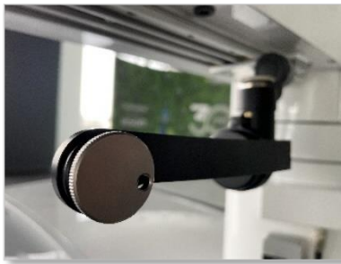
Figure 2: (De-) Mounting of the C-eye device by turning the dial (a) at the C-eye support (b) to (un-)fasten the C-eye device (c).
