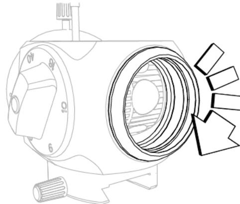
Fig. 166 - Screw in the lens
