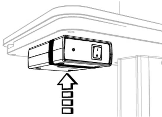
Fig. 25 - Place the power supply unit
