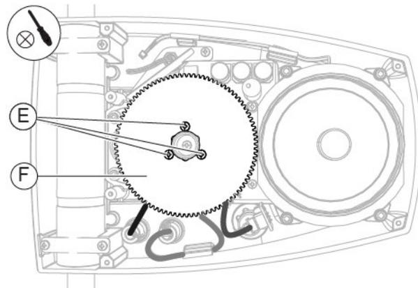
Fig. 373 - Place the cogwheel and screw in the screws
