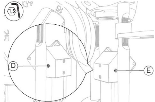
Fig. 382 - Loosen the screws
