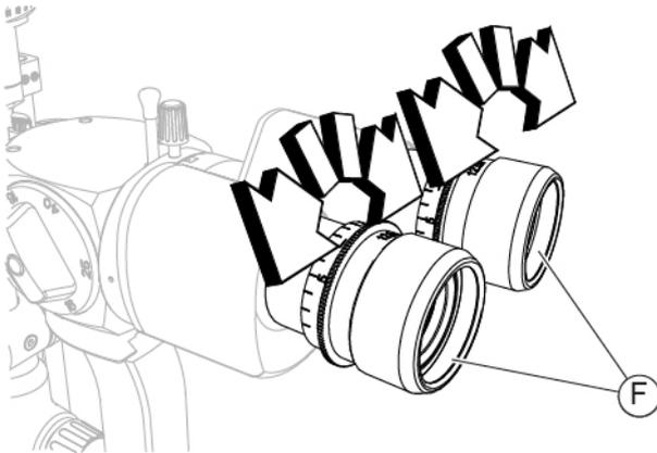
Fig. 152 - Turn the eyepiece with reference cross
