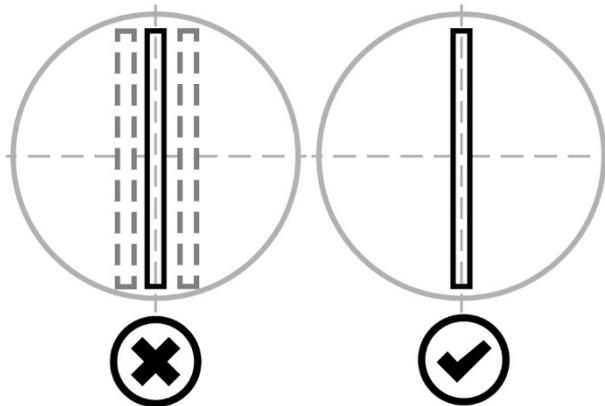
Fig. 353 - Check the vertical projection of the slit
