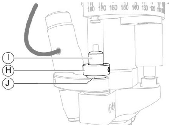
Fig. 240 - Remove the locking ring and the round ring
