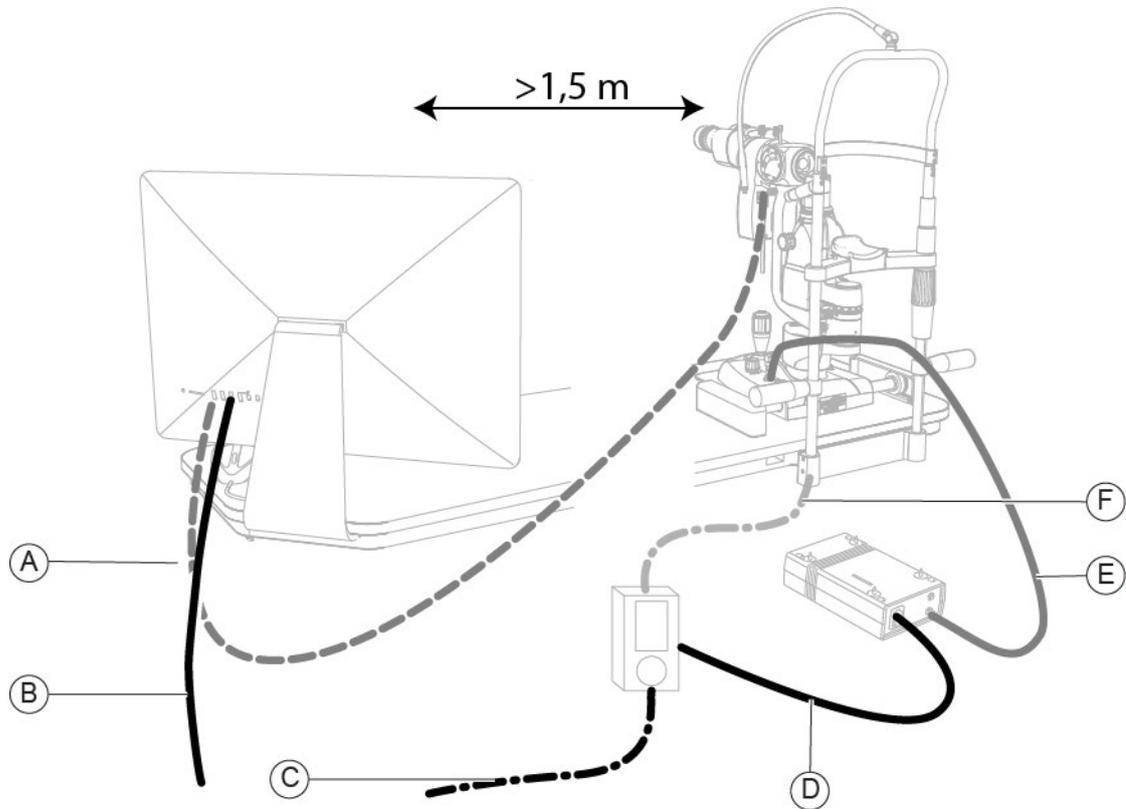
Fig. 391 - Connecting the tester outside the patient area
