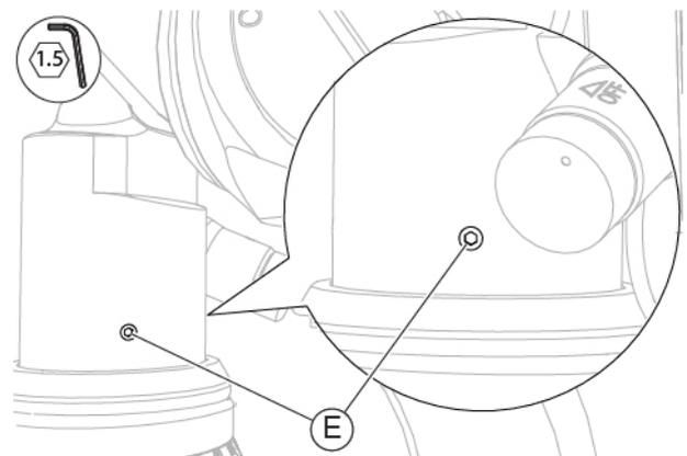
Fig 358 - Slightly loosen the screws
