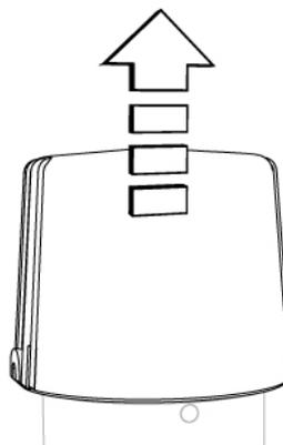
Fig. 201 - Remove the cover
