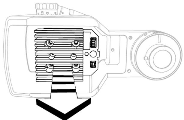
Fig. 184 - Remove the lighting unit
