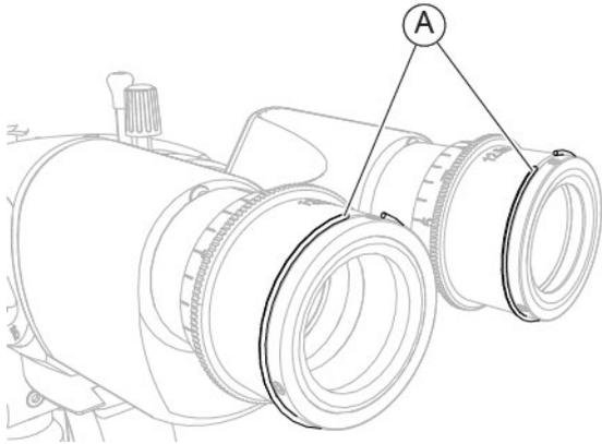
Fig. 106 - Install the sealing rings
