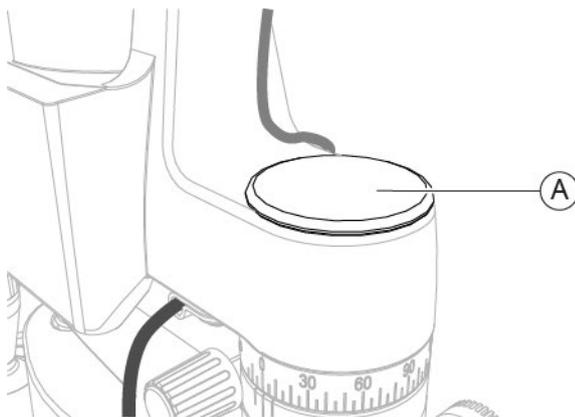
Fig. 56 - Remove the cap
