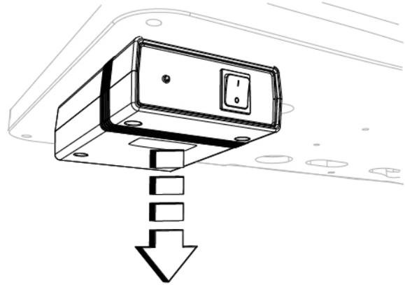
Fig. 100 - Remove the power supply unit
