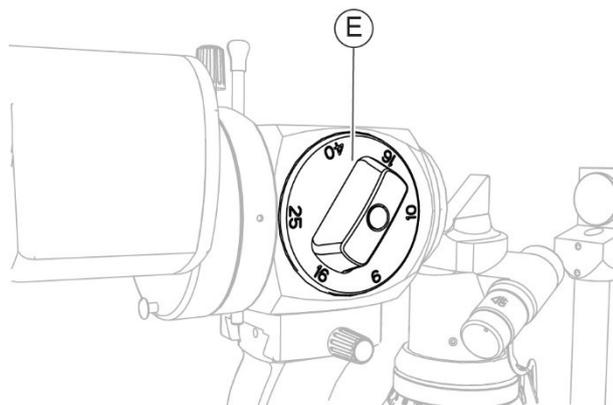
Fig. 59 - Turn the magnification adjuster selector
