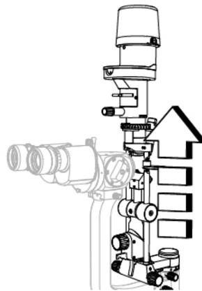
Fig. 365 - Remove the lighting assembly
