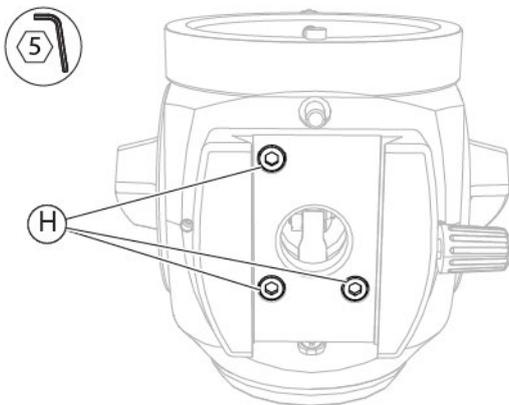
Fig. 154 - Loosen the screws
