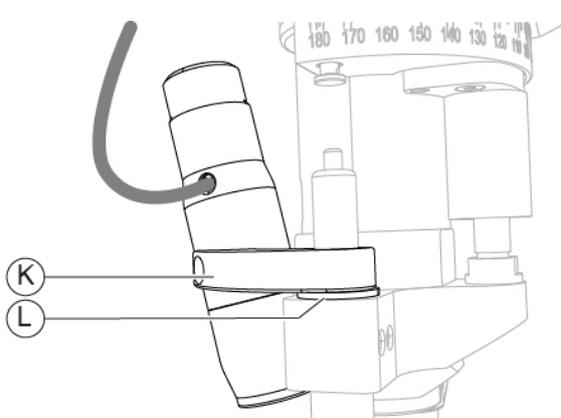
Fig. 243 - Insert the flat ring and the illuminator
