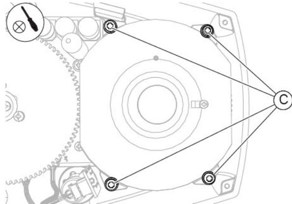
Fig. 285 - Screw in the screws
