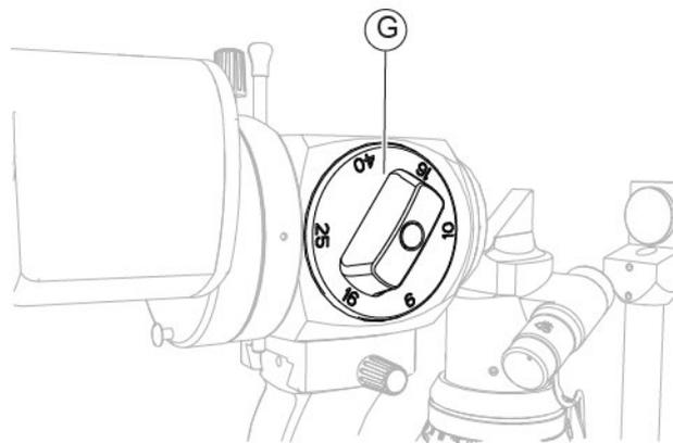
Fig. 141 - Turn the magnification adjuster selector
