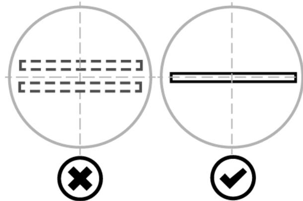
Fig. 386 - Check the horizontal projection of the slit
