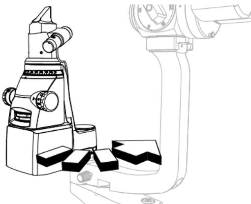
Fig. 197 - Turn the lighting assembly
