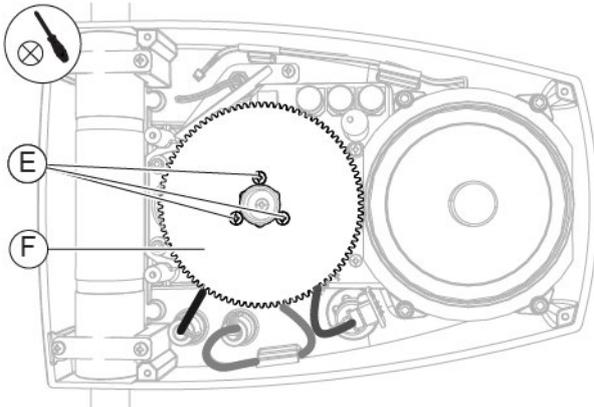
Fig. 366 - Unscrew the screws and remove the cogwheel
