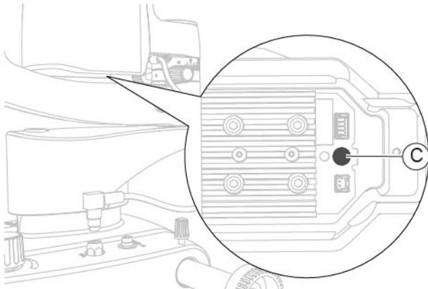
Fig. 71 - Light indicator of the lighting assembly
