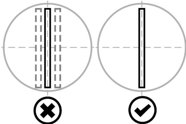
Fig. 95 - Check the vertical projection of the slit
