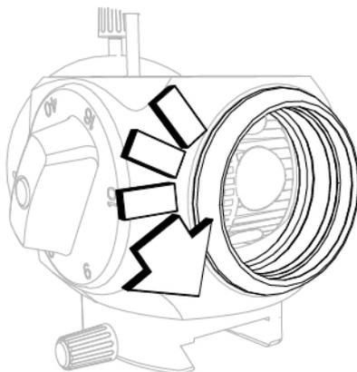
Fig. 165 - Unscrew and remove the lens
