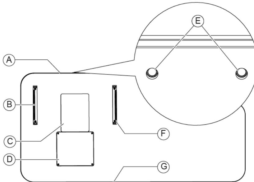
Fig. 21 - Installation accessories on the table top
