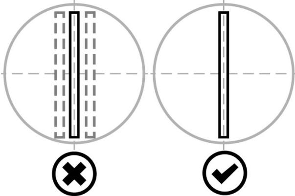
Fig. 82 - Check the vertical projection of the slit
