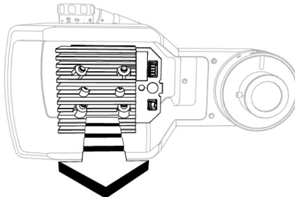
Fig. 307 - Remove the lighting unit
