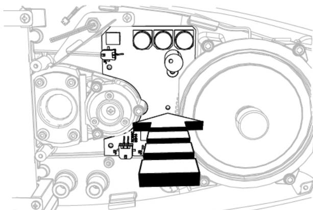
Fig. 210 – Place the circuit board
