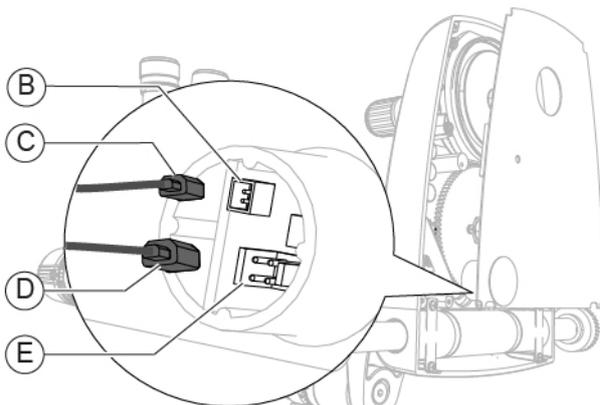
Fig. 270 - Disconnect the cables
