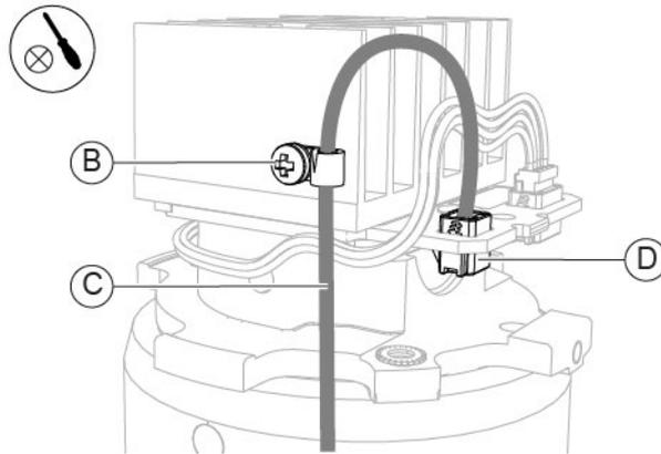
Fig. 247 – Connect the cable and screw in the screw
