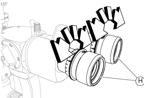
Fig. 93 - Turn the eyepiece with reference cross
