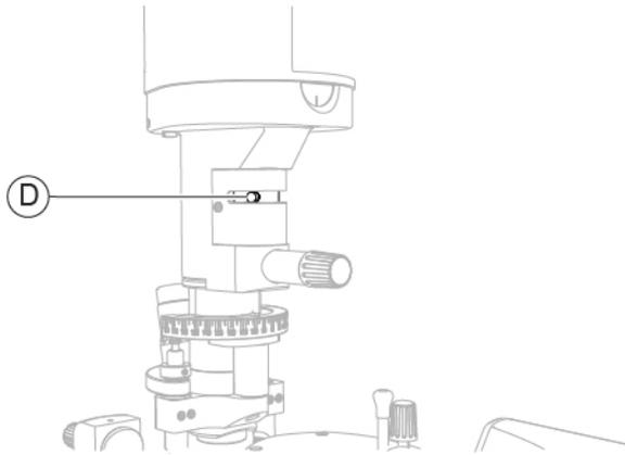
Fig. 89 - Turn the filter selector
