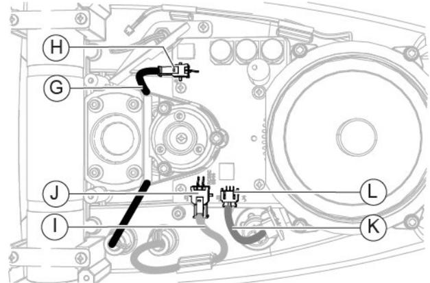
Fig. 367 - Disconnect the connection cables from the connectors
