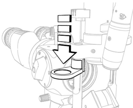
Fig. 251 - Lower the light diffusing filter
