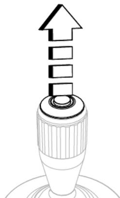
Fig. 295 - Remove the joystick button
