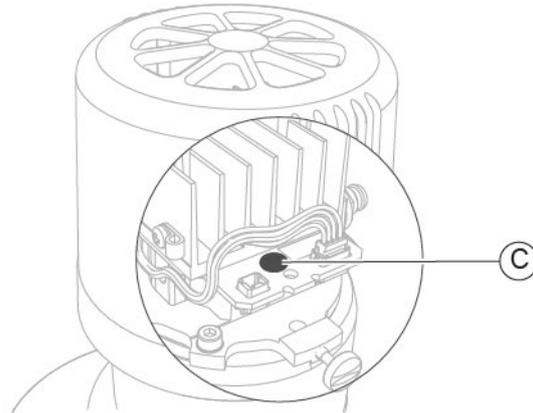
Fig. 72 - Light indicator of the lighting assembly
