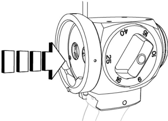
Fig. 126 - Install the binoculars
