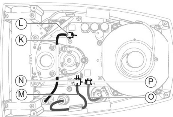
Fig. 191 - Connect the connection cables to the connectors
