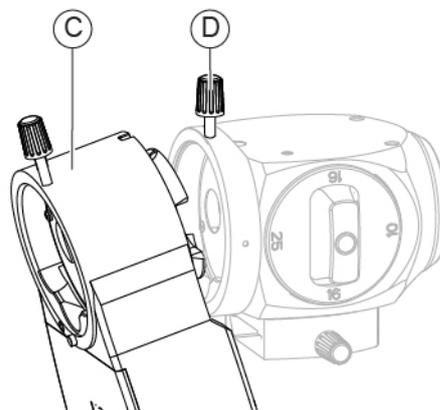
Fig. 119 - Remove the beam splitter
