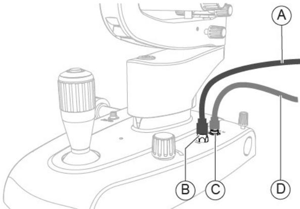
Fig. 336 - Disconnect the cables
