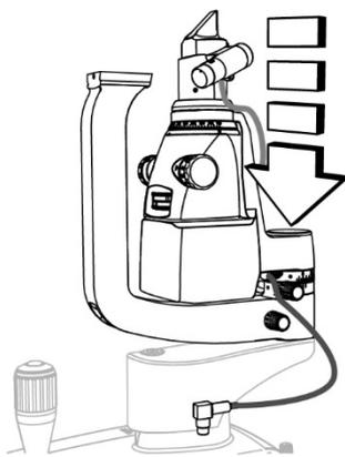
Fig. 347 - Place the lighting assembly complete with arm
