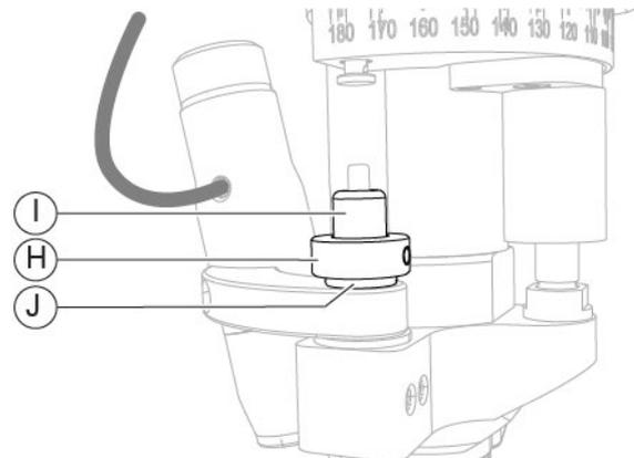
Fig. 244 - Insert the round ring and the locking ring
