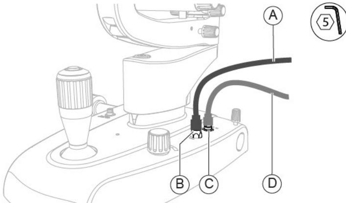
Fig. 317 - Disconnect the cables
