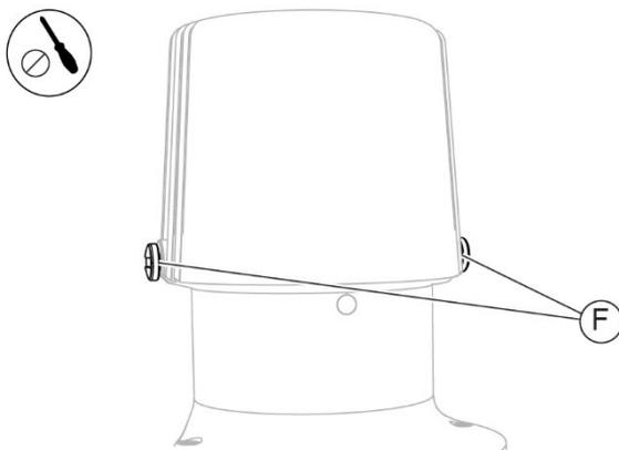
Fig. 320 - Unscrew the screws
