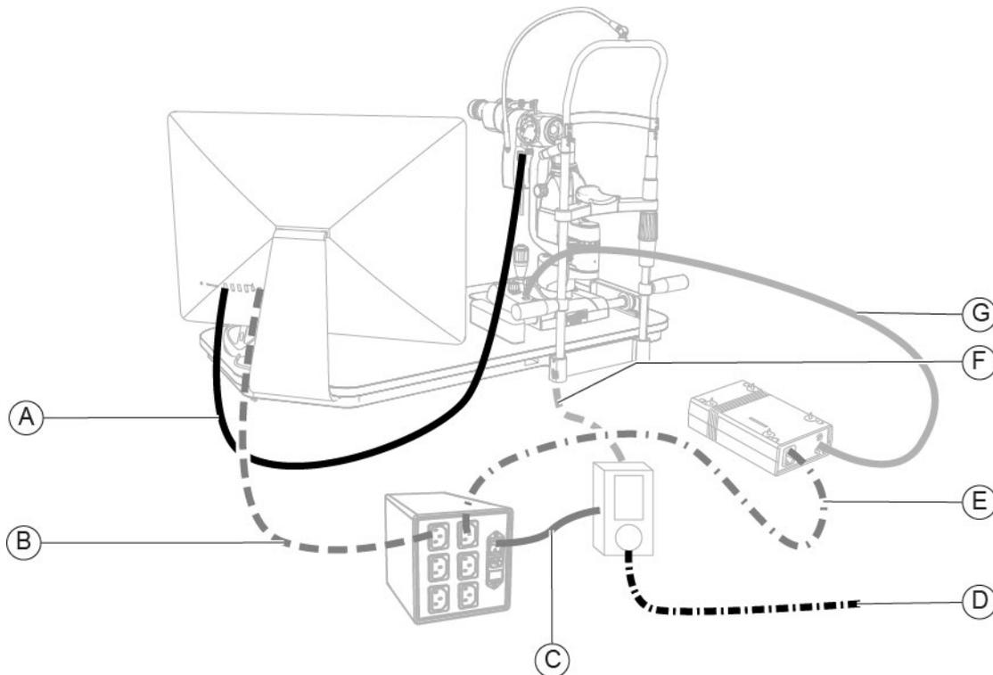
Fig. 390 - Connect the tester inside the patient area
