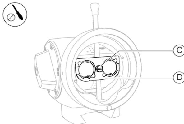
Fig. 169 - Remove the yellow filter
