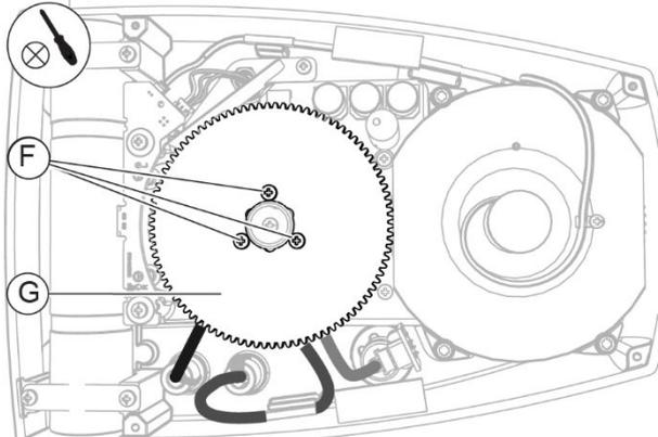
Fig. 339 - Unscrew the screws and remove the cogwheel
