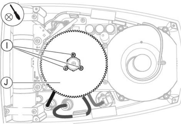
Fig. 185 - Unscrew the screws and remove the cogwheel
