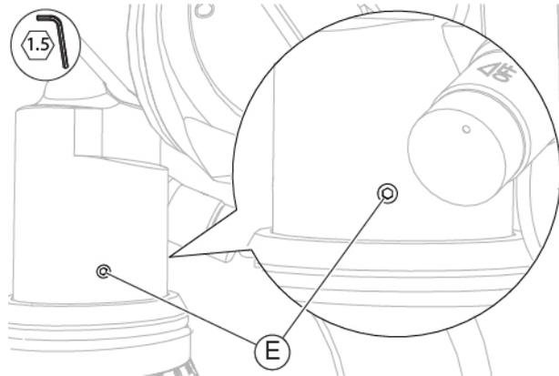
Fig. 360 - Tighten the screws
