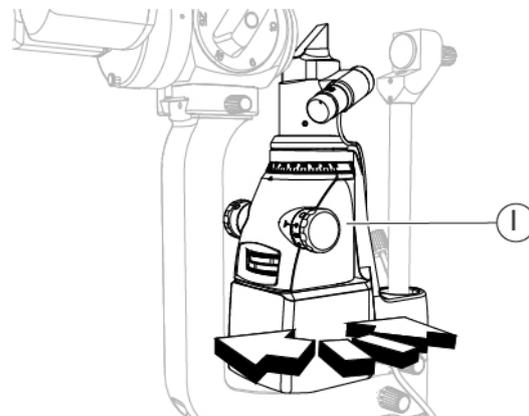
Fig. 81 - Swing the lighting assembly
