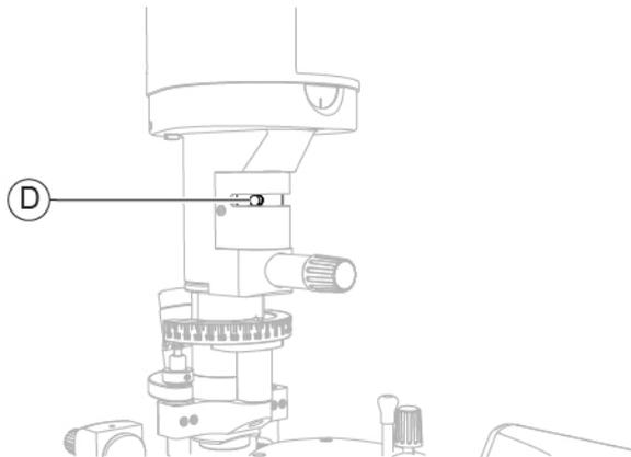
Fig. 150 - Turn the filter selector
