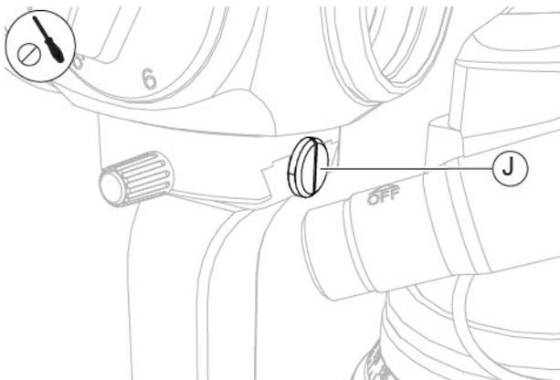
Fig. 140 - Loosen the stop element
