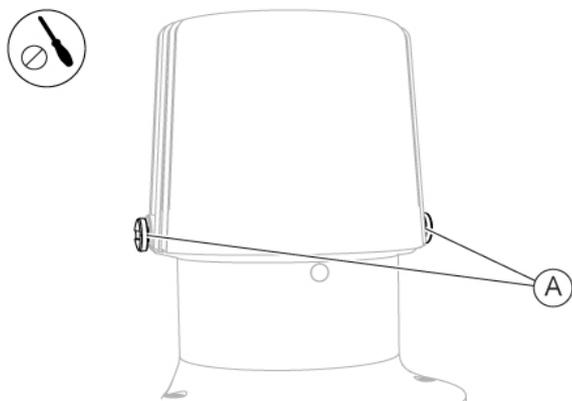
Fig. 200 - Unscrew the screws
