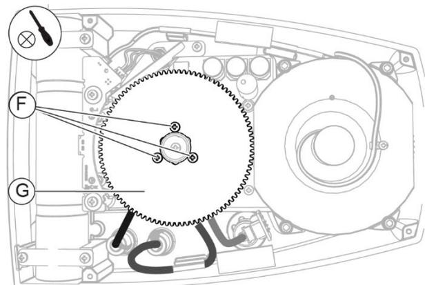
Fig. 346 - Place the cogwheel and screw in the screws
