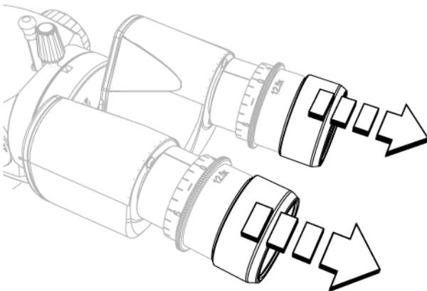
Fig. 104 - Remove the eyepiece covers
