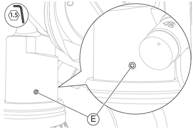
Fig. 354 - Slightly loosen one of the two screws
