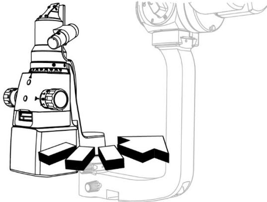
Fig. 312 - Turn the lighting assembly
