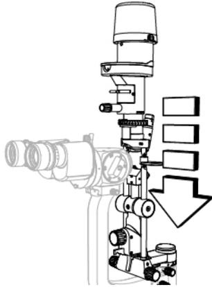
Fig. 374 - Place the lighting assembly
