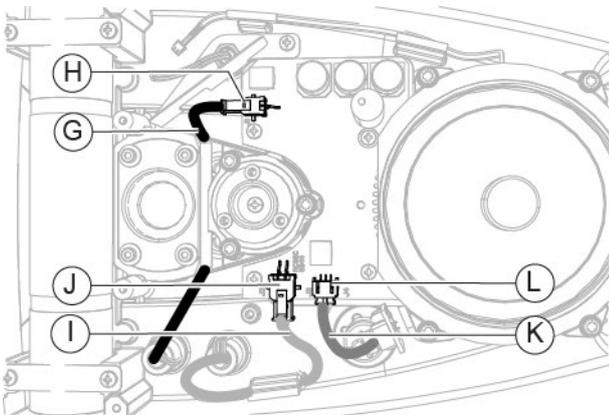
Fig. 372 - Connect the connection cables to the connectors
