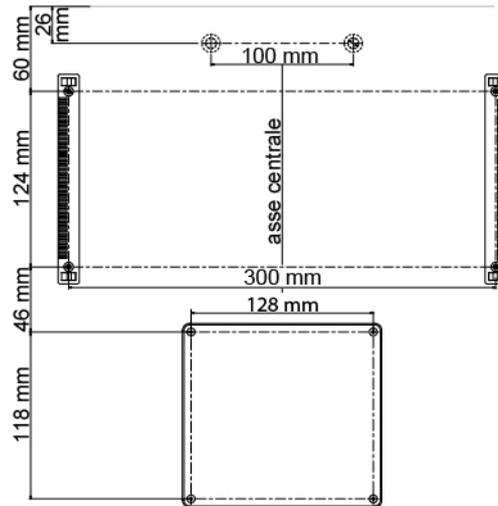
Fig. 22 - Distances for installation on the table top
