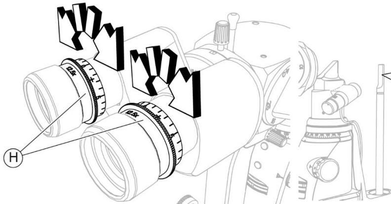
Fig. 62 - Turn the adjustment dial
