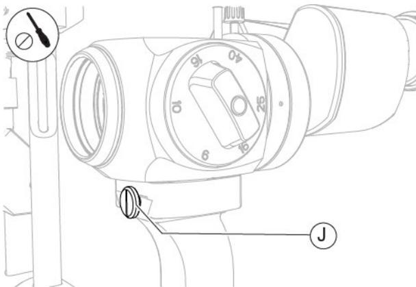
Fig. 158 - Loosen the stop element
