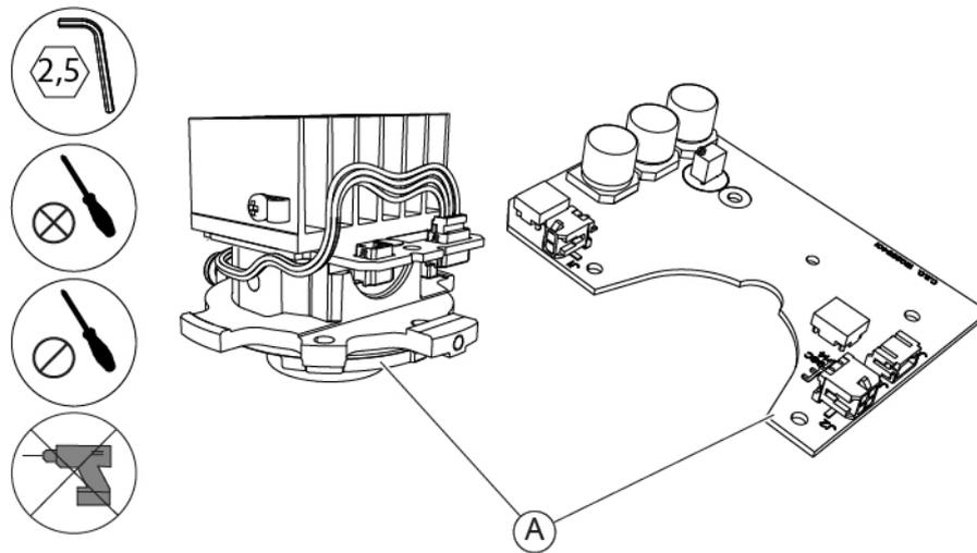
Fig. 199 - Lighting unit and circuit board
