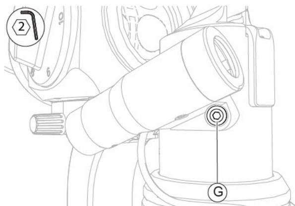
Fig. 225 - Unscrew the screw
