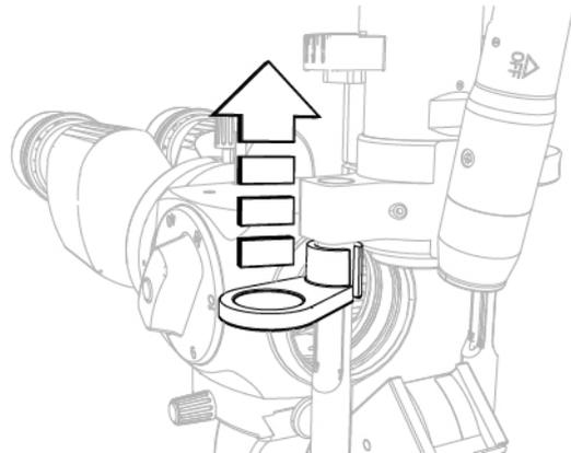
Fig. 254 - Lift the light diffusing filter
