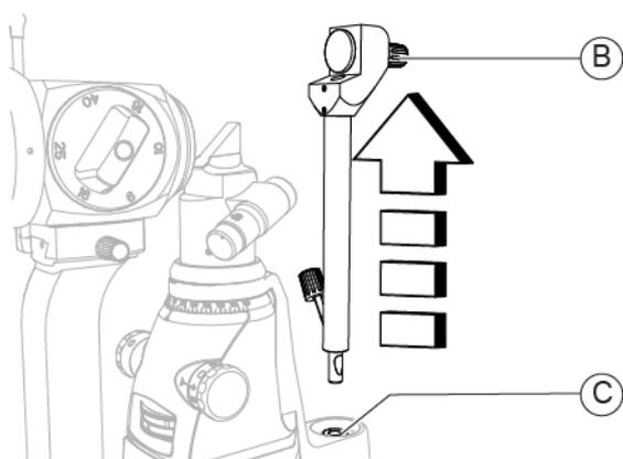
Fig. 145 - Remove the calibration rod
