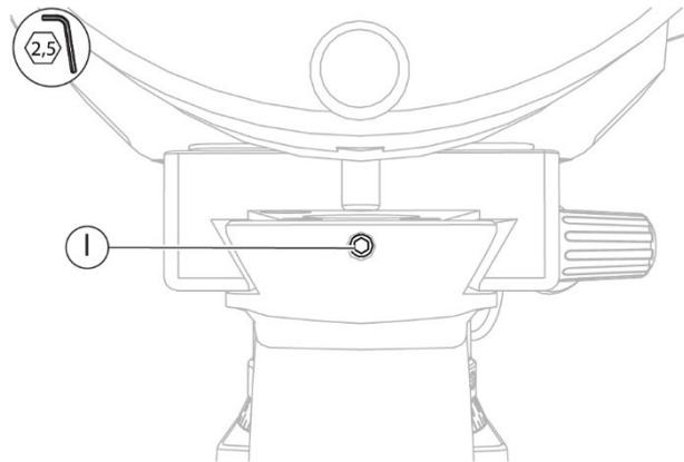
Fig. 139 - Loosen the screw
