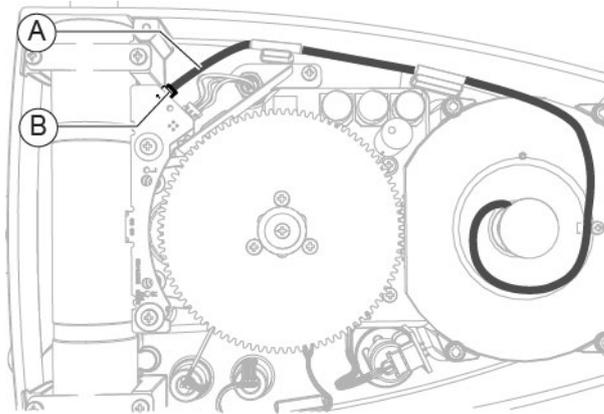
Fig. 286 - Connect the cable
