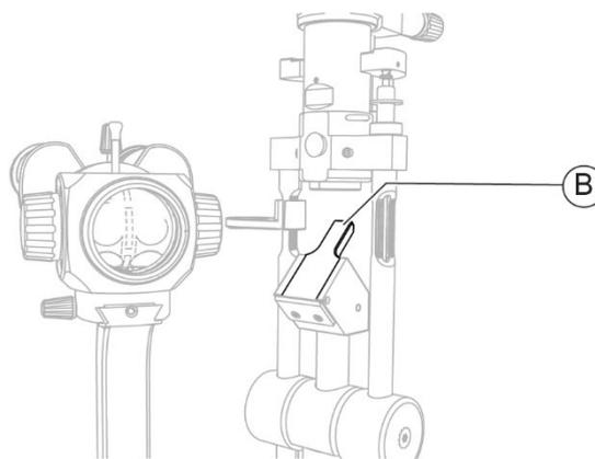
Fig. 175 - Remove the projection mirror
