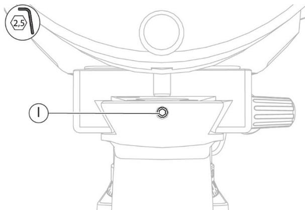
Fig. 144 - Tighten the screw
