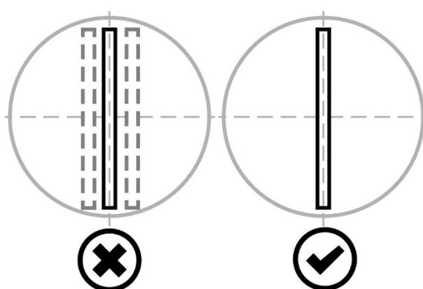
Fig. 381 - Check the vertical projection of the slit
