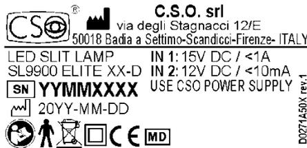
Fig. 7 - Data plate for the Xx-D model
