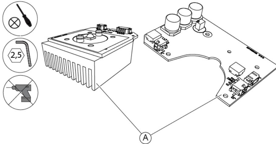
Fig. 178 - Lighting unit and circuit board
