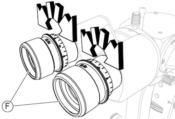
Fig. 134 - Turn the eyepiece with reference cross
