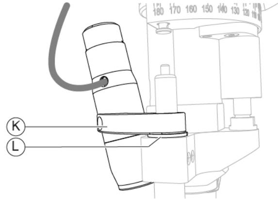
Fig. 241 - Remove the illuminator and the flat ring
