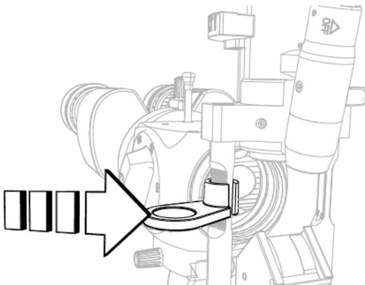
Fig. 253 - Insert the light diffusing filter
