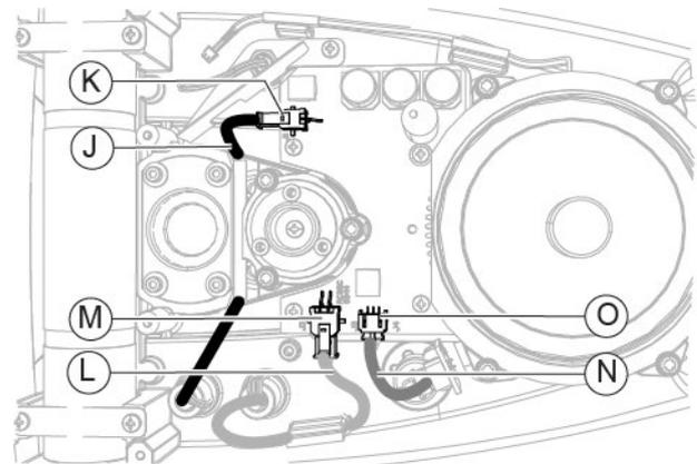
Fig. 207 - Disconnect the cables from the connectors
