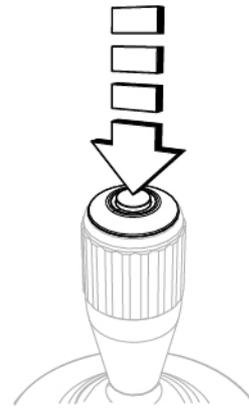
Fig. 298 - Insert the joystick button
