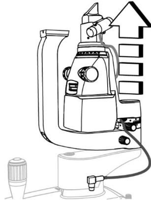
Fig. 338 - Remove the lighting assembly complete with arm
