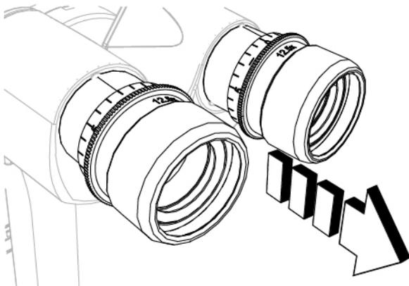
Fig. 109 - Remove the eyepieces
