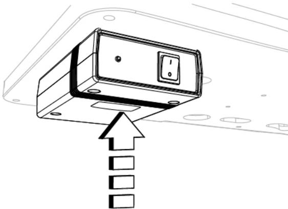
Fig. 101 - Place the power supply unit
