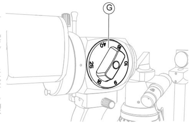
Fig. 135 - Turn the magnification adjuster selector
