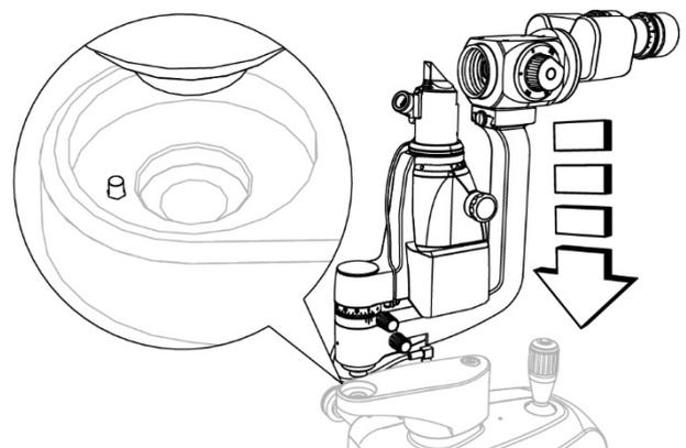
Fig. 313 - Insert the structure assembly complete with lighting assembly
