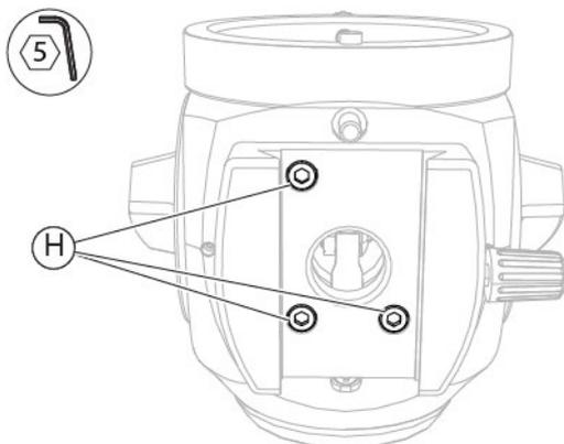
Fig. 136 - Loosen the screws
