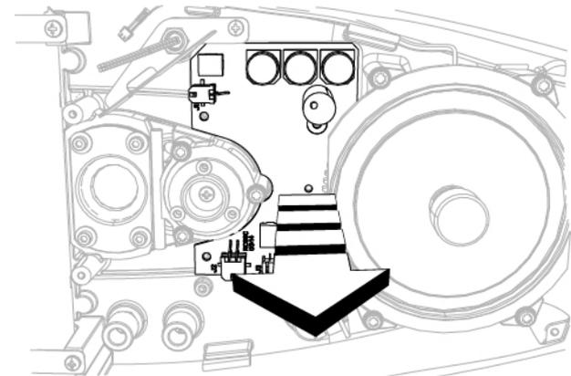
Fig. 209 - Remove the circuit board
