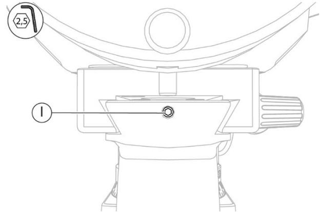
Fig. 157 - Loosen the screw
