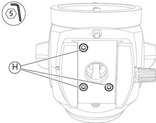
Fig. 156 - Tighten the screws
