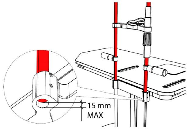
Fig. 32 - Maximum adjustment height of the rods
