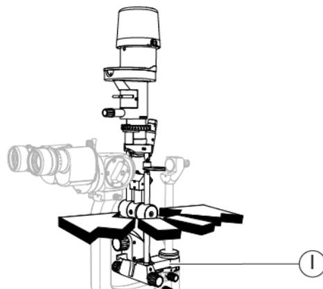
Fig. 94 - Swing the lighting assembly
