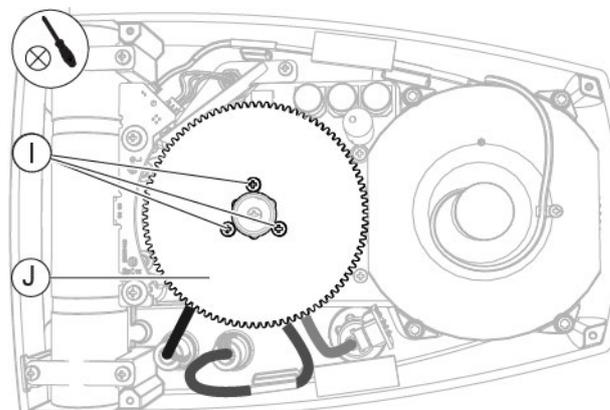
Fig. 192 - Place the cogwheel and screw in the screws
