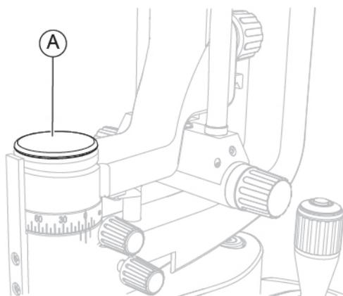
Fig. 87 - Remove the cap
