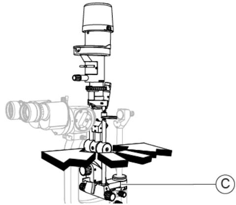
Fig. 380 - Swing the lighting assembly
