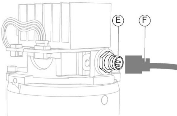
Fig. 216 - Connect the cable
