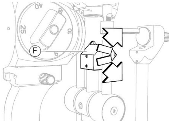
Fig. 388 - Tilting of the reflection mirror assembly
