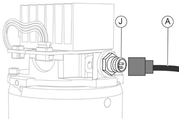
Fig. 323 - Disconnect the cable
