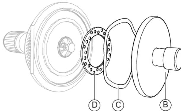
Fig. 290 - Remove the disc, the gasket and the bearing
