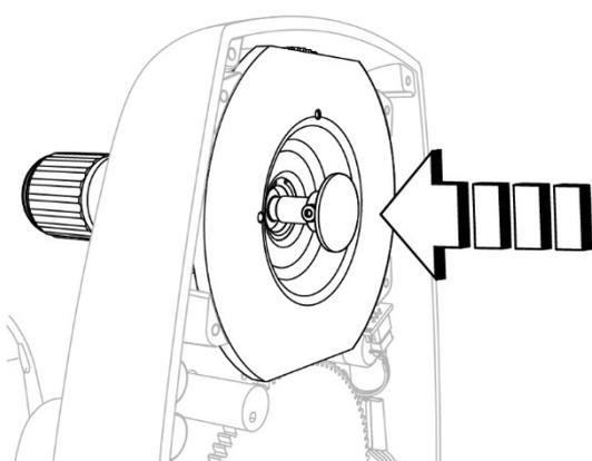
Fig. 278 - Insert the joystick
