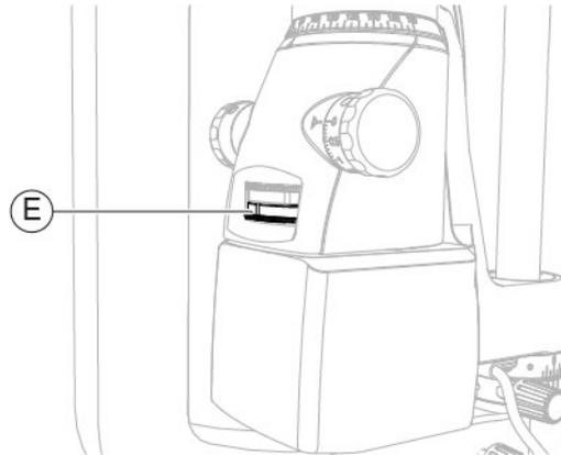
Fig. 133 - Turn the filter selector
