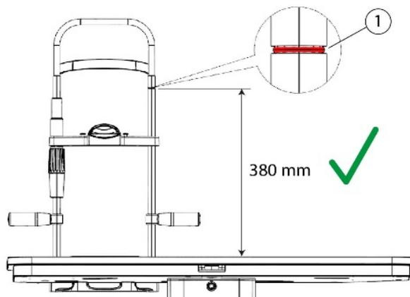
Fig. 30 - Correct height of the eye level indicator
