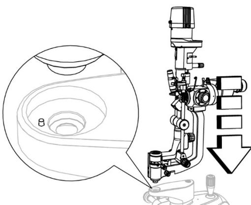
Fig. 332 - Insert the structure assembly complete with lighting assembly
