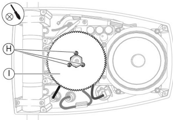
Fig. 206 - Unscrew the screws and remove the cogwheel
