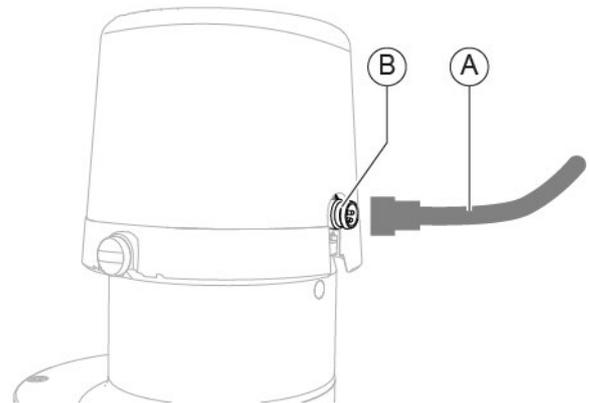
Fig. 377 - Connect the cable
