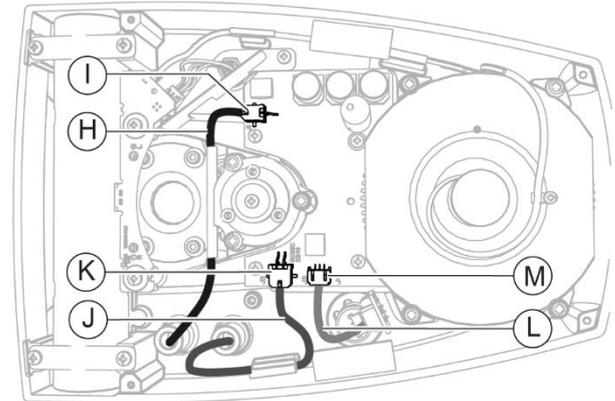
Fig. 340 - Disconnect the connection cables from the connectors
