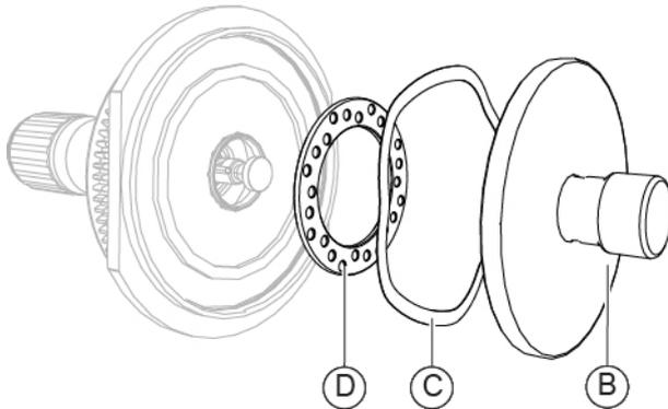
Fig. 291 - Insert the bearing, the gasket and the disc
