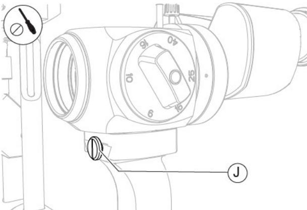
Fig. 160 - Tighten the stop element
