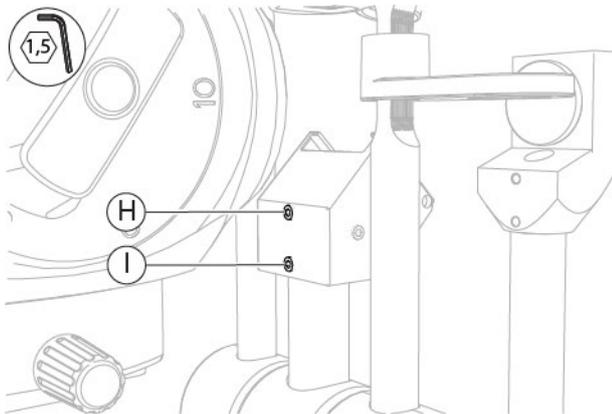
Fig. 387 - Adjust the screws
