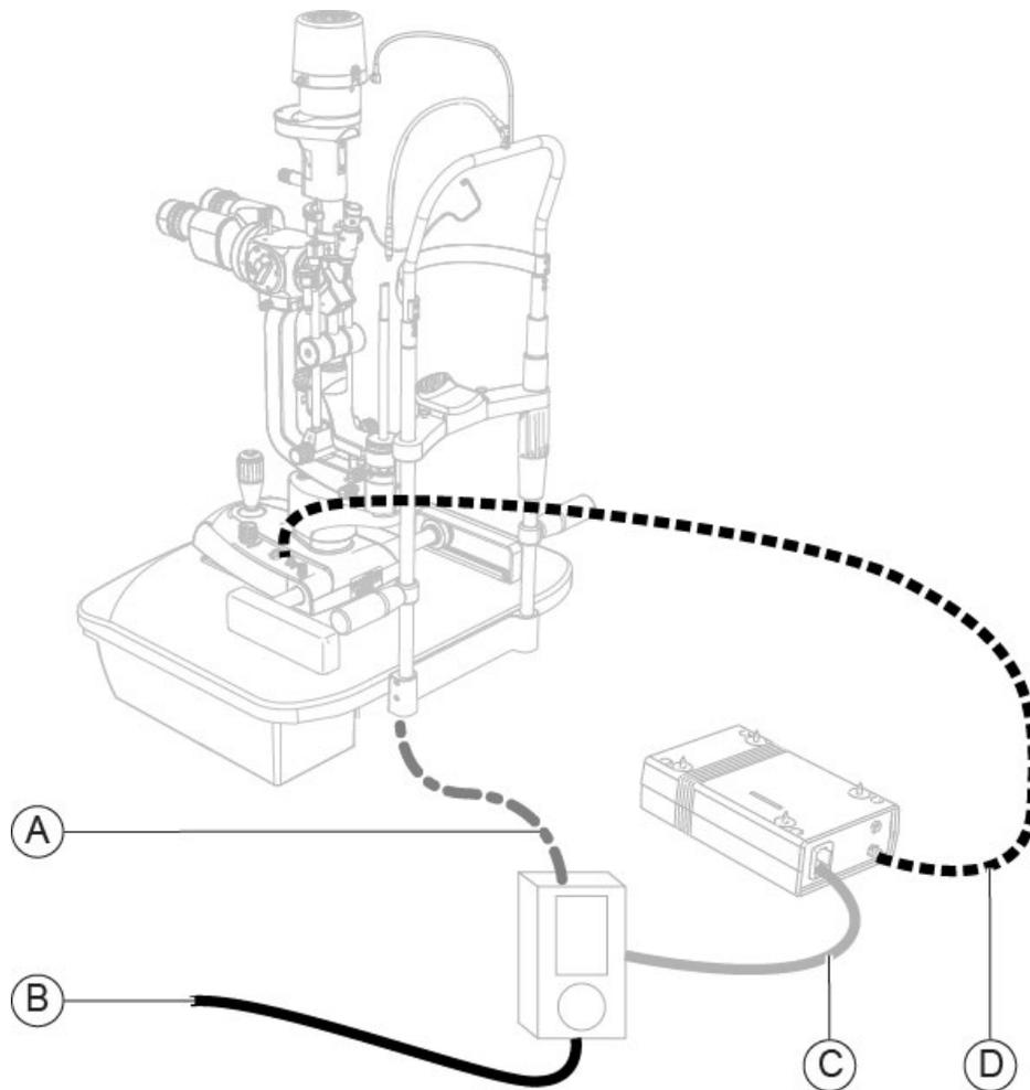
Fig. 392 - Connect the tester
