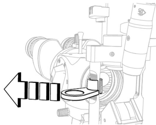
Fig. 252 - Remove the light diffusing filter
