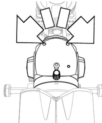
Fig. 155 - Turn the magnification adjuster
