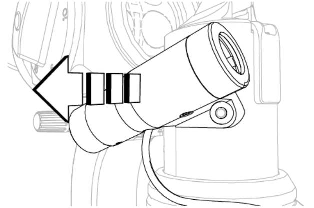
Fig. 226 - Remove the illuminator
