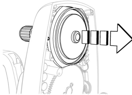
Fig. 289 - Remove the joystick
