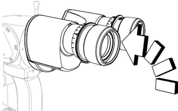
Fig. 114 - Place the binoculars
