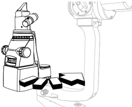
Fig. 231 - Turn the lighting assembly
