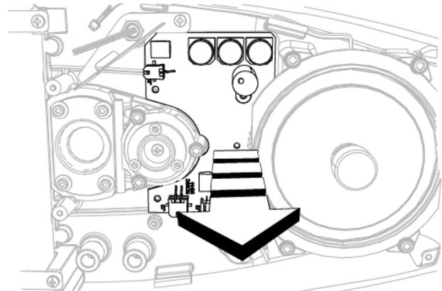
Fig. 369 - Remove the circuit board
