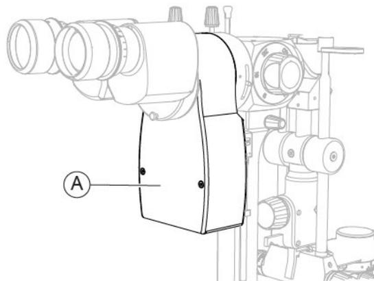
Fig. 116 - Beam splitter
