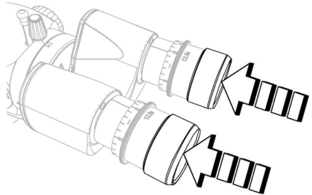
Fig. 107 - Install the eyepiece covers
