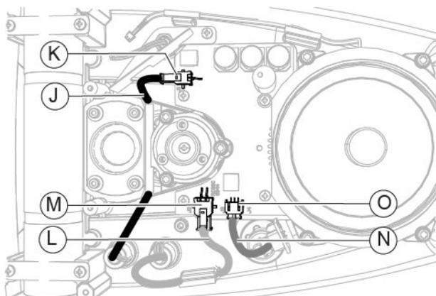
Fig. 212 - Connect the cables to the connectors
