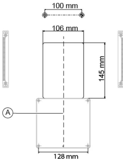
Fig. 23 - Distances for installing the sticker pad
