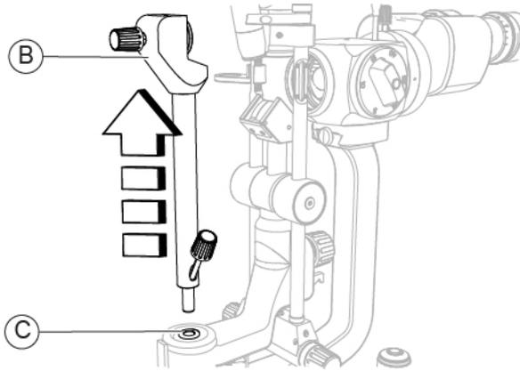
Fig. 162 - Remove the calibration rod
