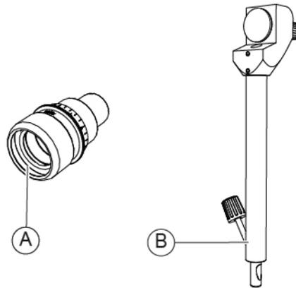
Fig. 86 - Eyeiece with reference cross and calibration rod
