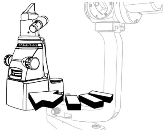
Fig. 180 - Turn the lighting assembly
