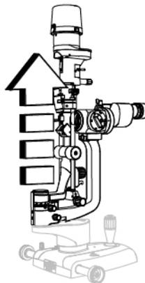
Fig. 319 - Remove the structure assembly complete with lighting assembly
