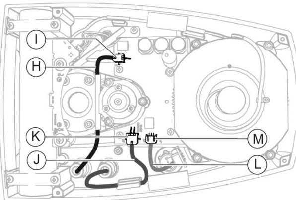
Fig. 345 - Connect the connection cables to the connectors
