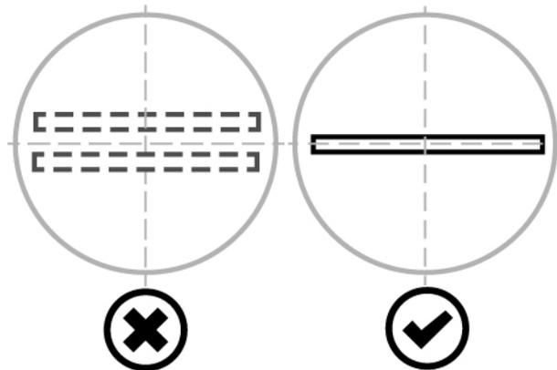
Fig. 85 - Check the horizontal projection of the slit
