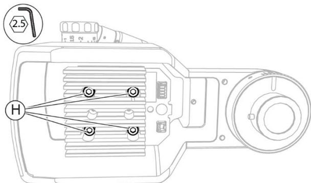
Fig. 306 - Unscrew the screws
