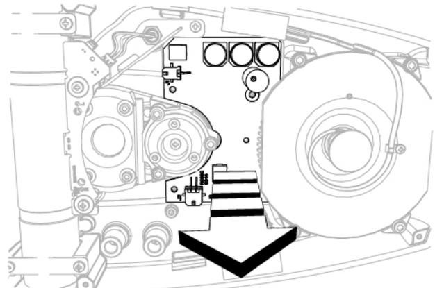
Fig. 342 - Remove the circuit board
