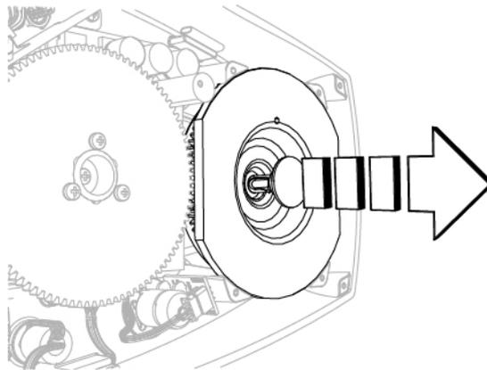
Fig. 283 - Remove the joystick
