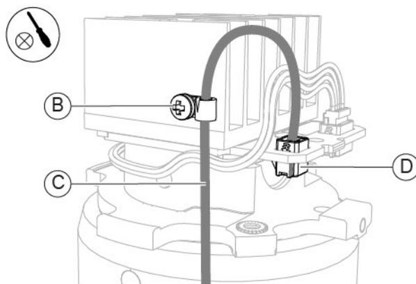
Fig. 236 - Unscrew the screw and disconnect the cable
