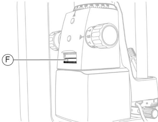
Fig. 60 - Turn the filter selector
