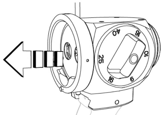
Fig. 125 - Remove the magnification adjuster
