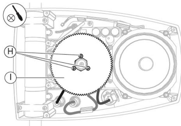
Fig. 213 - Place the cogwheel and screw in the screws
