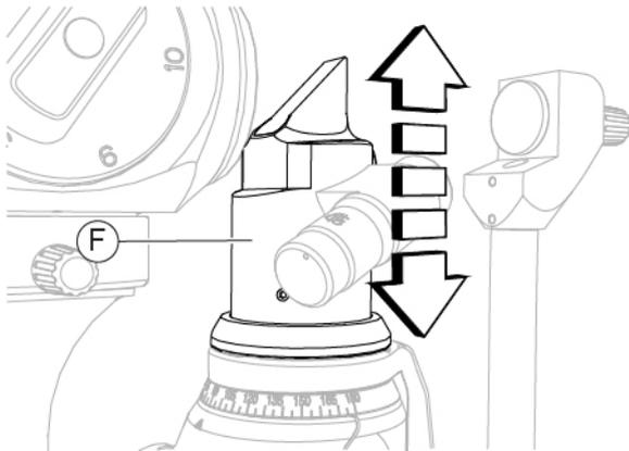
Fig. 359 - Move the prism-holder head
