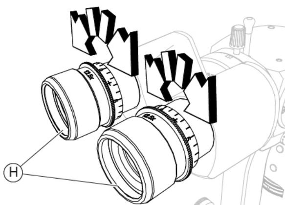
Fig. 80 - Turn the eyepiece with reference cross
