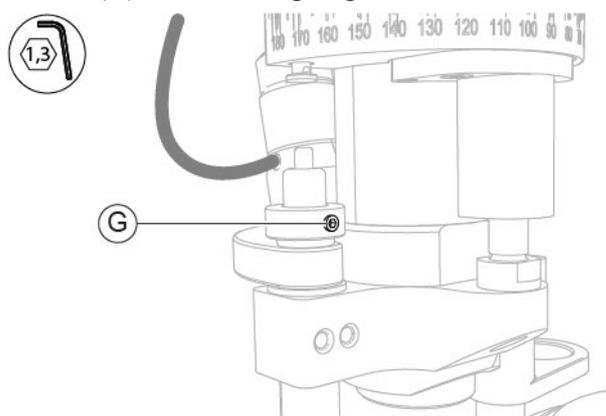
Fig. 239 - Unscrew the screw
