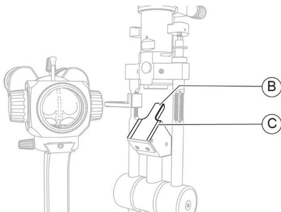
Fig. 176 - Insert the projection mirror
