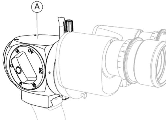
Fig. 123 - Magnification adjuster
