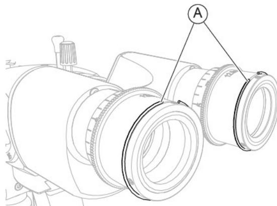
Fig. 105 - Remove the sealing rings
