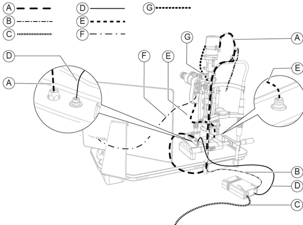
Fig. 36 - SL9900 and SL9900 ELITE connections [Digital configuration]
