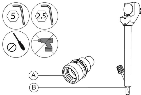
Fig. 147 - Eyepiece with reference cross and calibration rod
