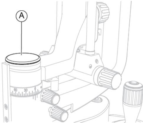
Fig. 148 - Remove the cap
