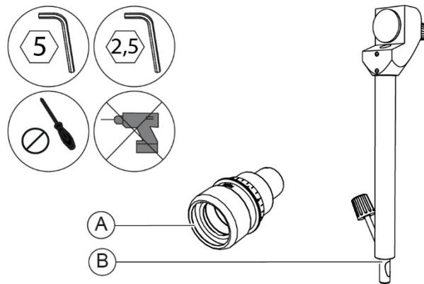
Fig. 129 - Eyepiece with reference cross and calibration rod
