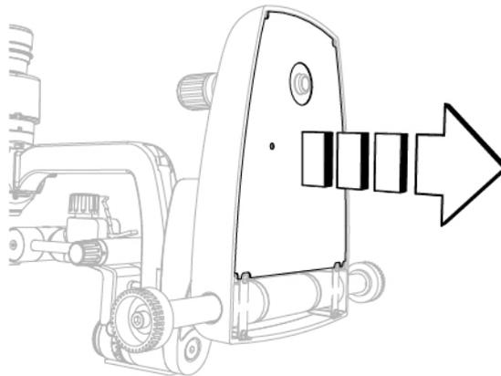
Fig. 258 - Remove the plate
