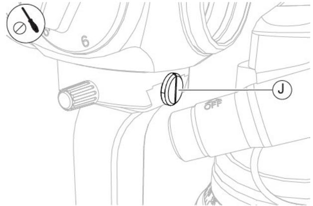
Fig. 143 - Tighten the stop element
