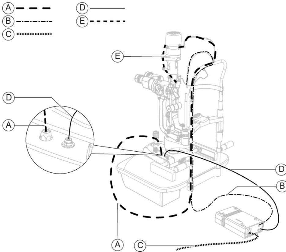
Fig. 35 - SL9900 connections [Standard configuration]
