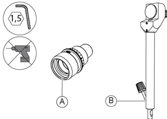
Fig. 350 - Eyepiece with reference cross and calibration rod
