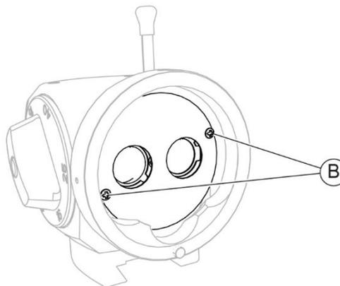
Fig. 172 - Place the plate and screw in the screws
