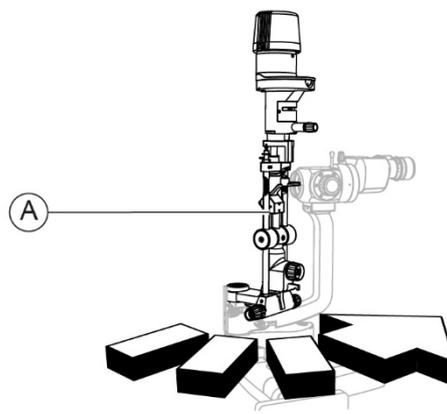
Fig. 177 - Turn the lighting assembly
