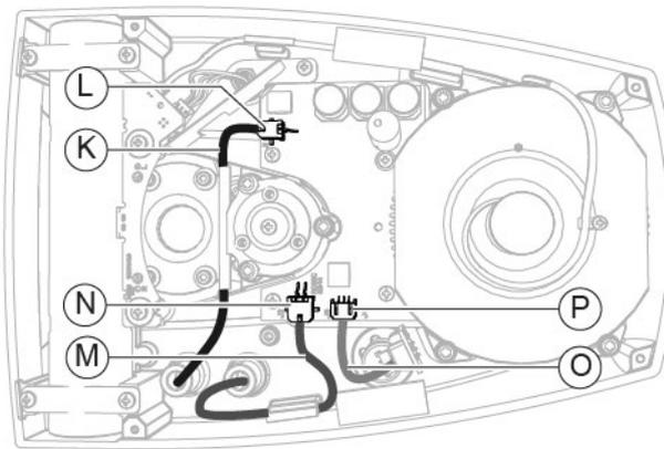
Fig. 186 - Disconnect the connection cables from the connectors
