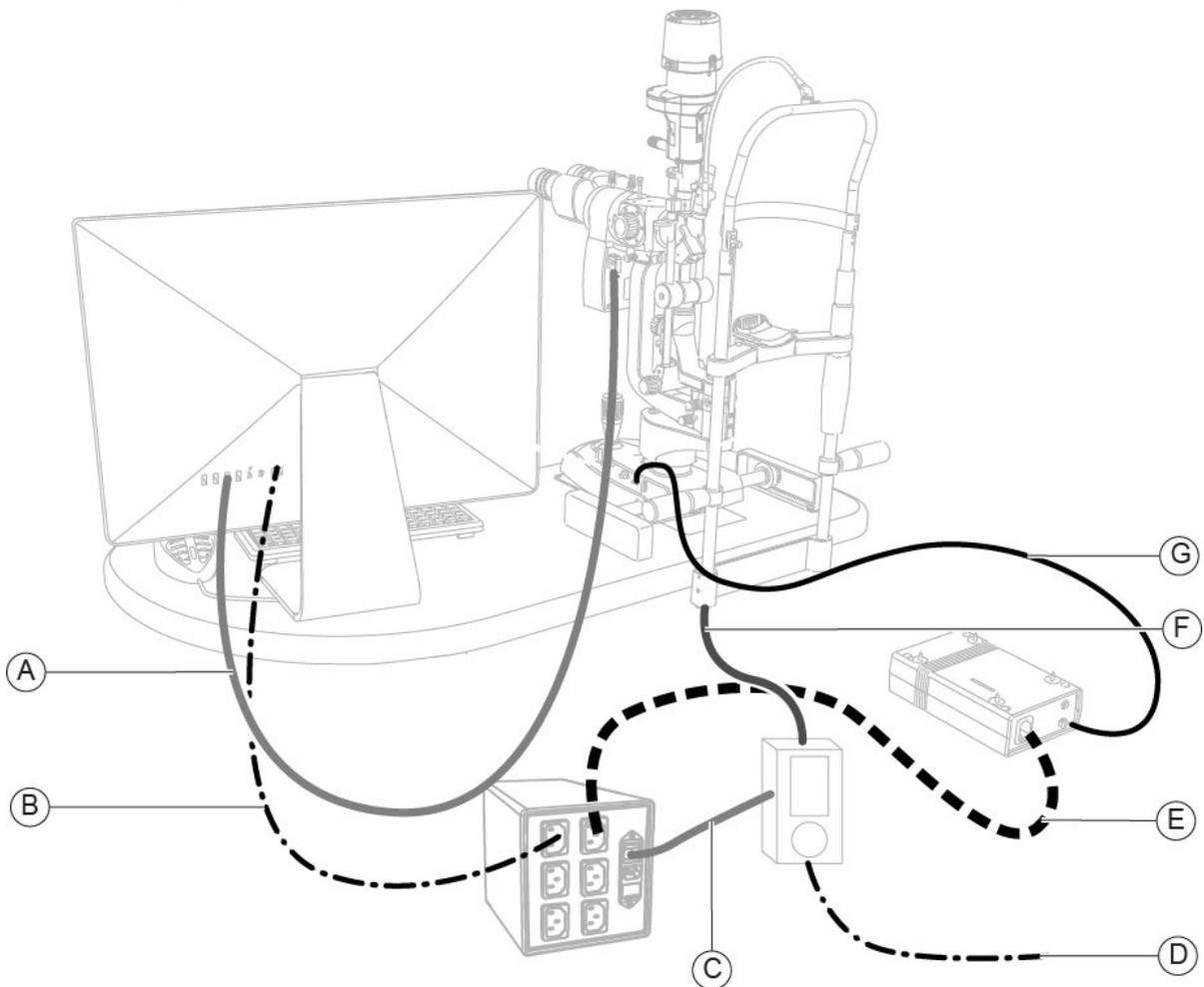
Fig. 393 - Connect the tester inside the patient area
