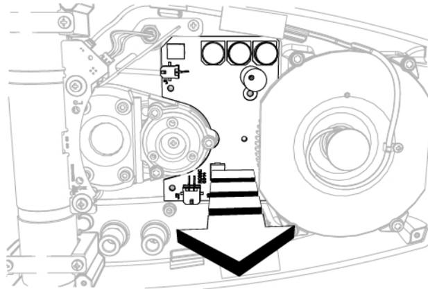
Fig. 188 - Remove the circuit board
