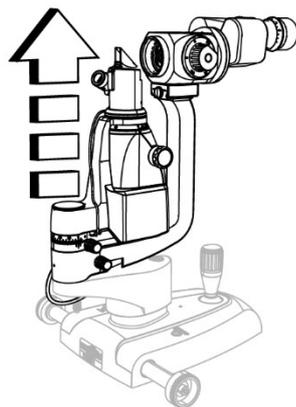
Fig. 302 - Remove the structure assembly complete with lighting assembly
