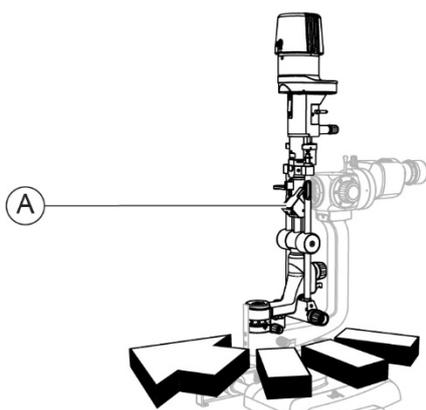
Fig. 174 - Turn the lighting assembly
