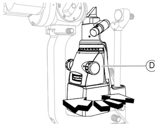
Fig. 352 - Swing the lighting assembly
