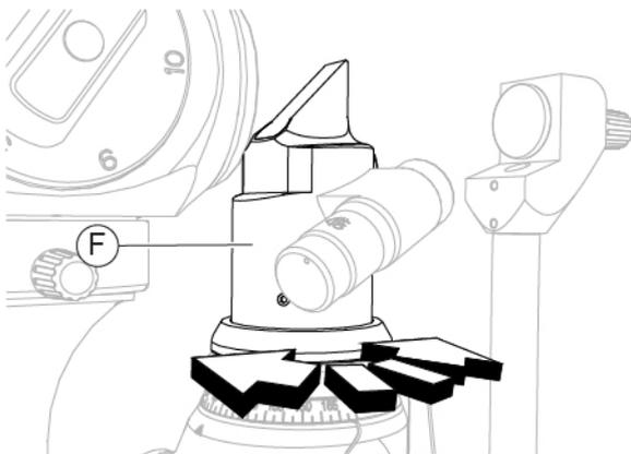
Fig. 355 - Turn the prism-holder head
