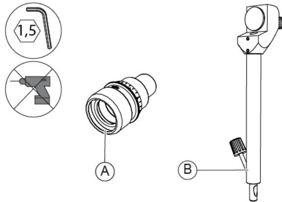
Fig. 378 - Eyepiece with reference cross and calibration rod
