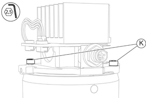
Fig. 324 - Unscrew the screws
