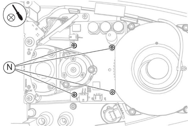
Fig. 344 - Screw in the screws
