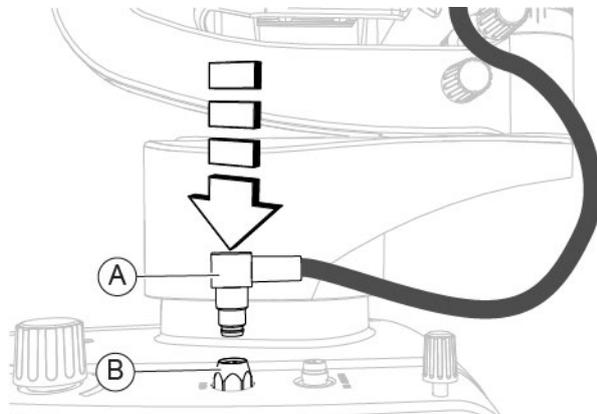
Fig. 198 - Connect the cable
