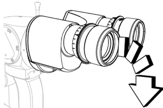
Fig. 113 - Remove the binoculars
