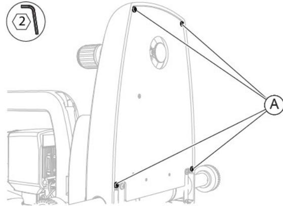
Fig. 263 - Unscrew the screws
