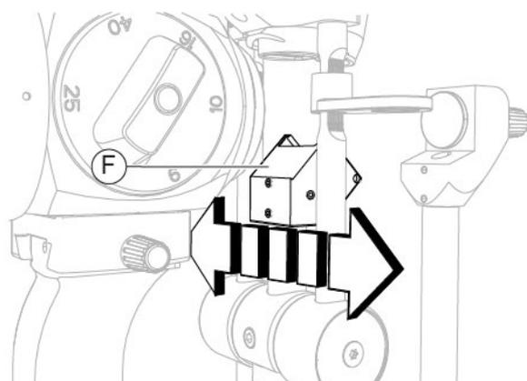
Fig. 383 - Move the reflection mirror assembly
