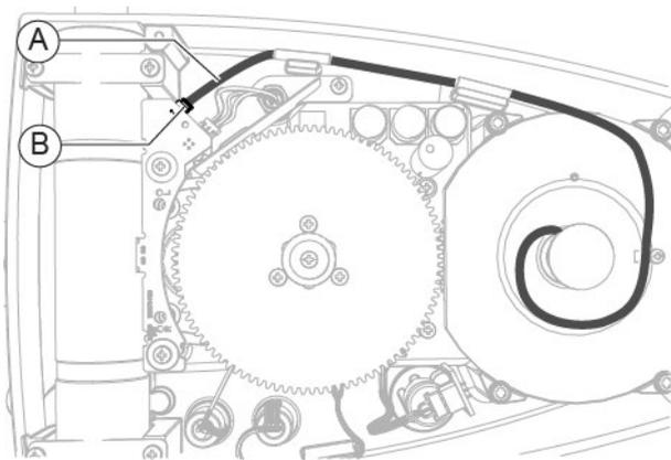
Fig. 281 - Disconnect the cable
