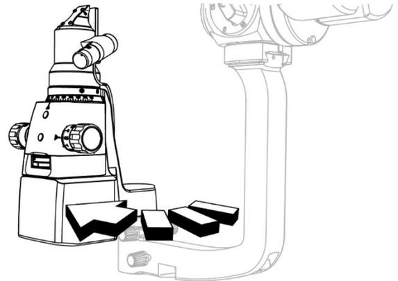
Fig. 303 - Turn the lighting assembly
