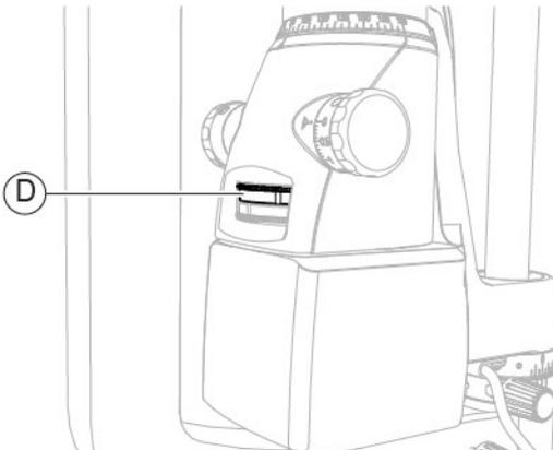
Fig. 132 - Turn the adjustment dial
