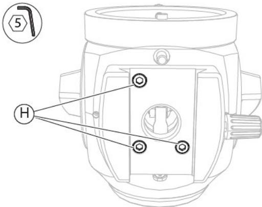
Fig. 138 - Tighten the screws
