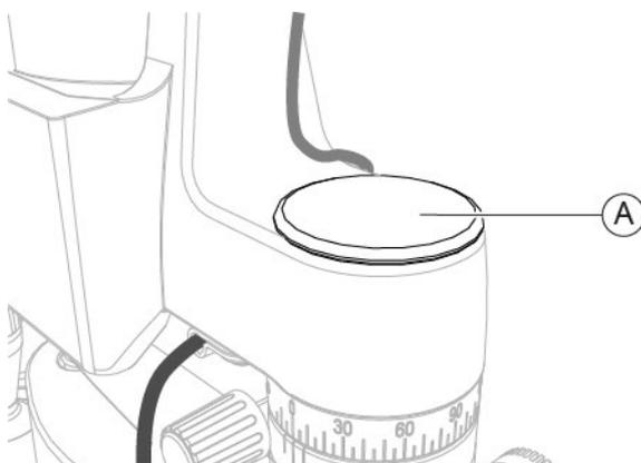
Fig. 74 - Remove the cap
