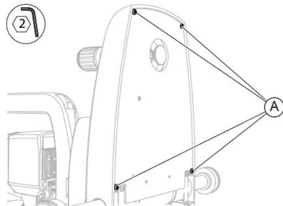
Fig. 266 - Screw the screws
