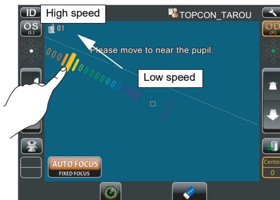
During vertical/lateral directions movement, the movement mode is changed to back /forth by tapping (at one second) the center of screen.
