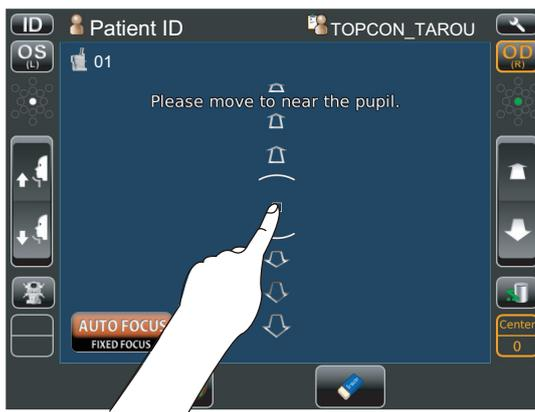
Under Back/forth movement mode, it is possible to move like the arrow of the screen.
