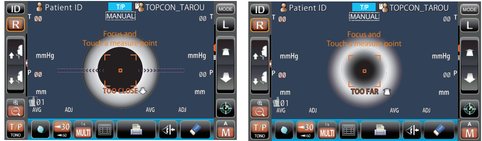
Limit of movement in the forward direction
