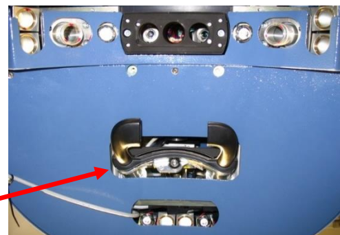
Figure 4-6: Particle Aspiration System
