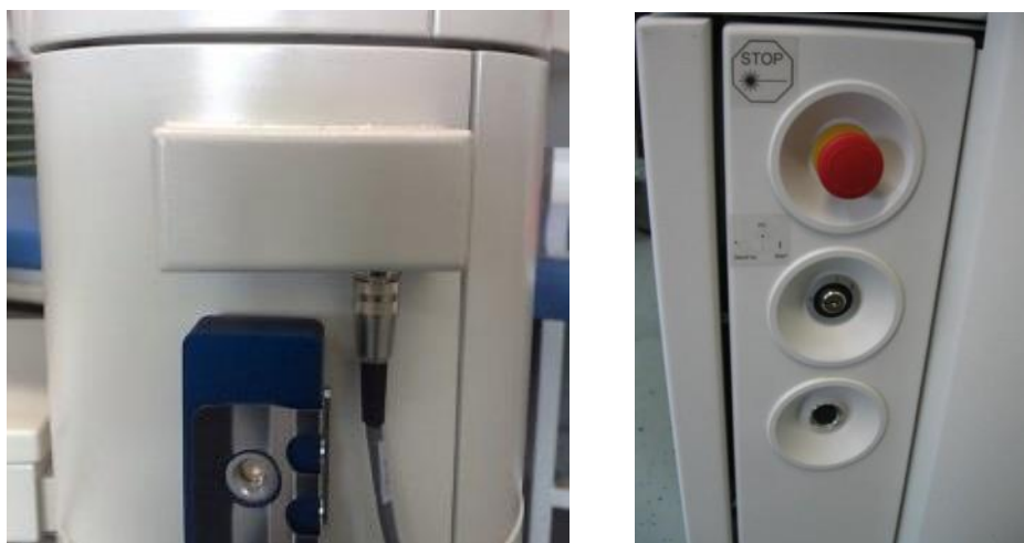
Figure 7-15: Connection of the fluence detector at AMARIS / AMARIS 750S/1050RS and AMARIS 500E
