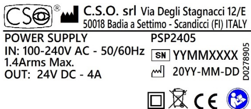
Fig. 3 - PSP2405 power supply unit data plate
