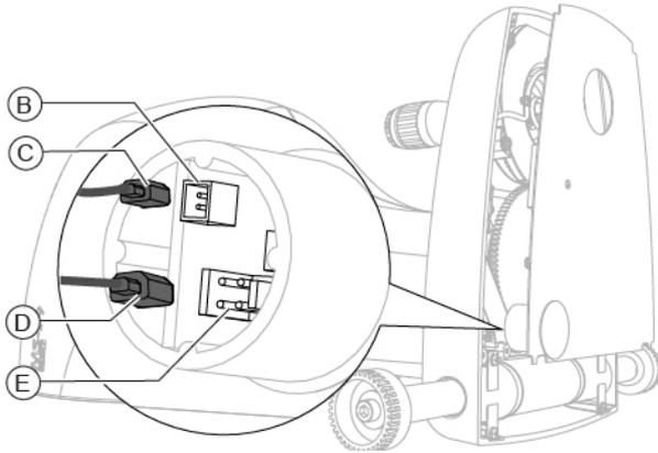
Fig. 75 - Disconnect the cables
