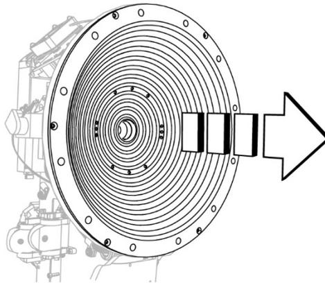
Fig. 71 - Remove the Placido disk
