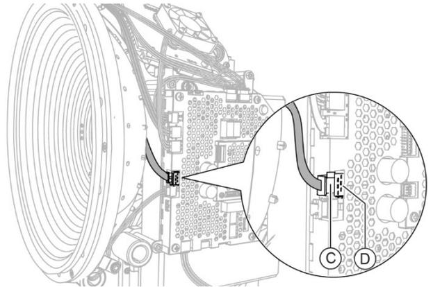
Fig. 70 - Disconnect the connection cable
