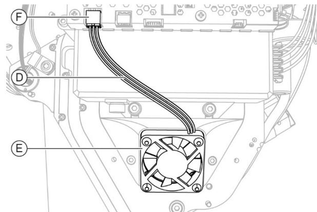
Fig. 92 - Disconnect the connection cable
