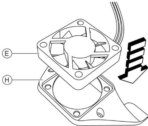
Fig. 95 - Place the fan on the support
