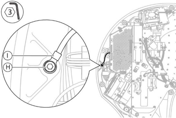
Fig. 66 - Unscrew the screw and disconnect the cable
