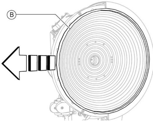
Fig. 60 - Remove the ring
