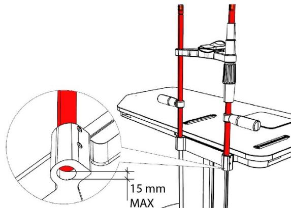
Fig. 20 - Maximum adjustment height of the rods
