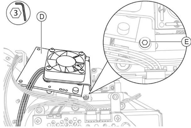
Fig. 110 - Place the assembly and screw in the screw
