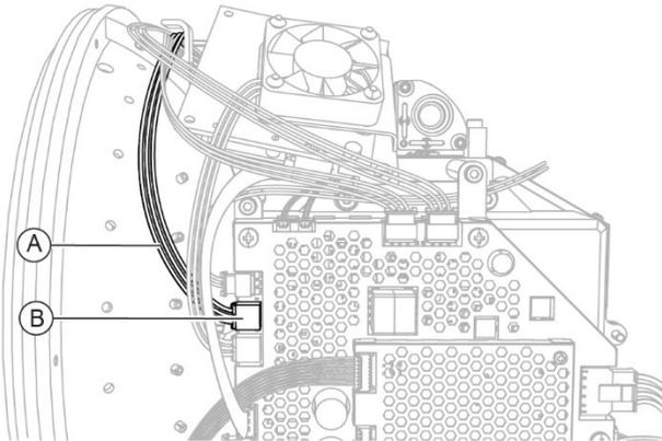
Fig. 113 - Disconnect the connection cable
