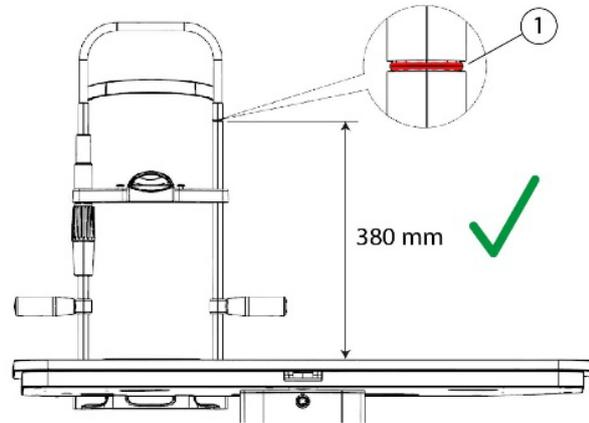
Fig. 18 - Correct height of the eye level indicator
