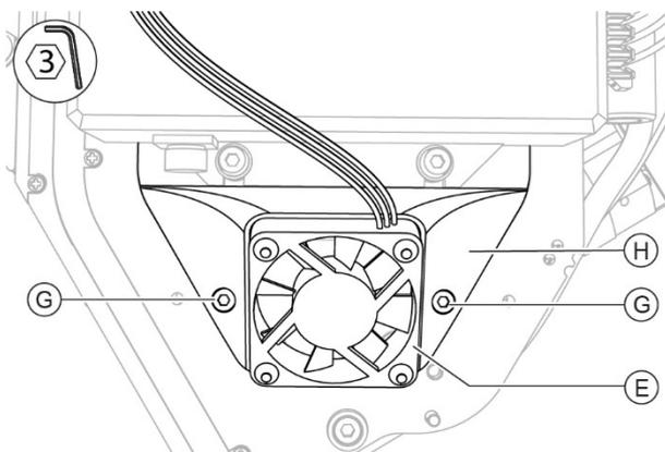
Fig. 93 - Remove the stand complete with cooling fan
