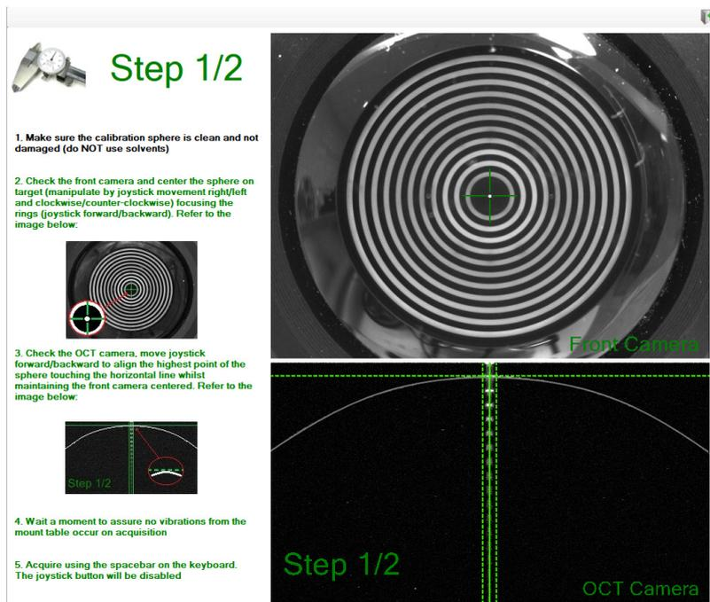
Fig. 51 - Curvature calibration Step 1/2
