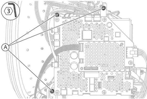
Fig. 89 - Loosen the screws
