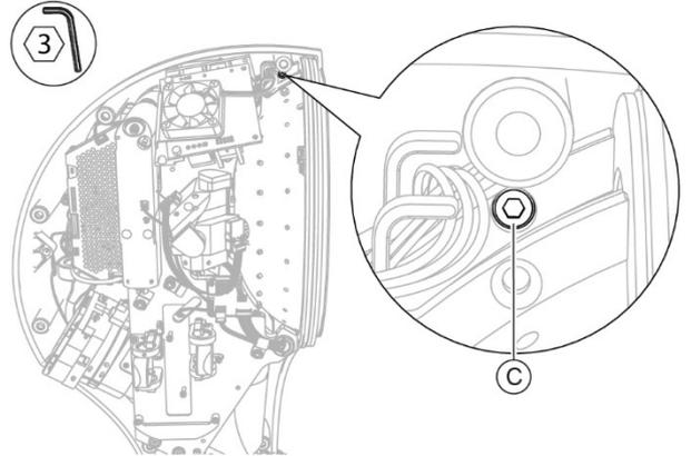
Fig. 61 - Unscrew the screw
