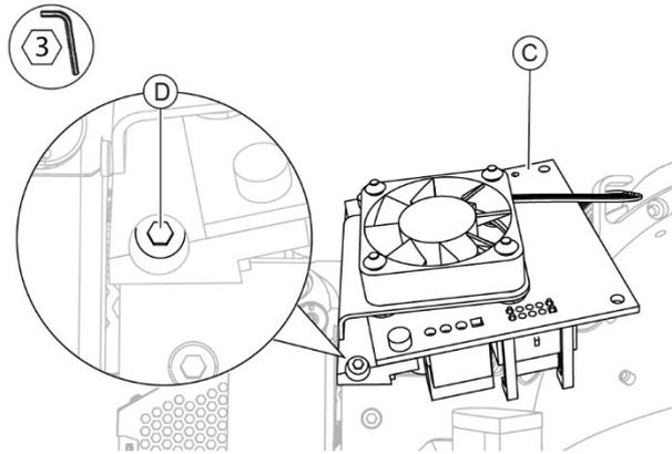
Fig. 114 - Unscrew the screw and remove the assembly
