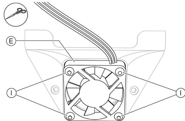
Fig. 94 - Cut the anti-vibration supports and remove the fan
