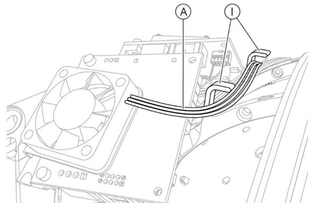
Fig. 120 - Pass the connection cable
