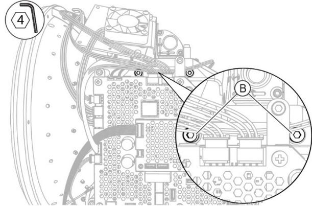
Fig. 100 - Tighten the screws
