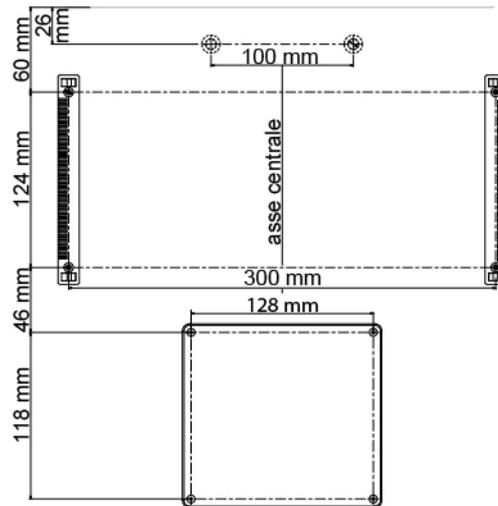
Fig. 11 - Distances for installation on the table top
