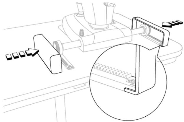
Fig. 16 - Install the wheel covers
