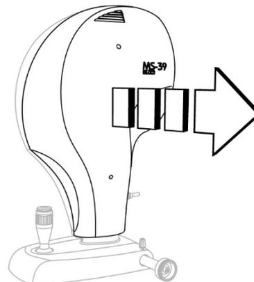
Fig. 59 - Remove the right protective shell
