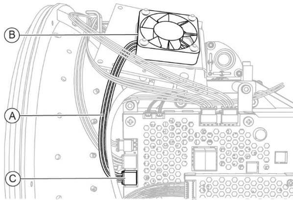
Fig. 111 - Connect the connection cable
