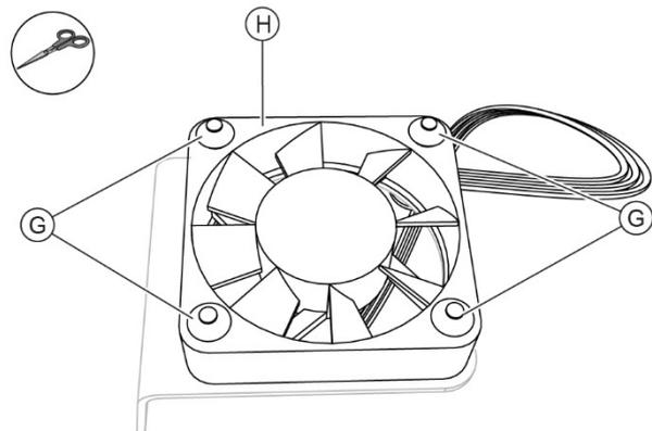
Fig. 116 - Cut the anti-vibration supports
