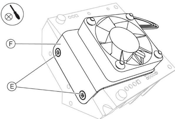
Fig. 115 - Unscrew the screws and remove the support
