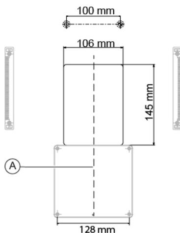
Fig. 12 - Distances for installing the sticker pad
