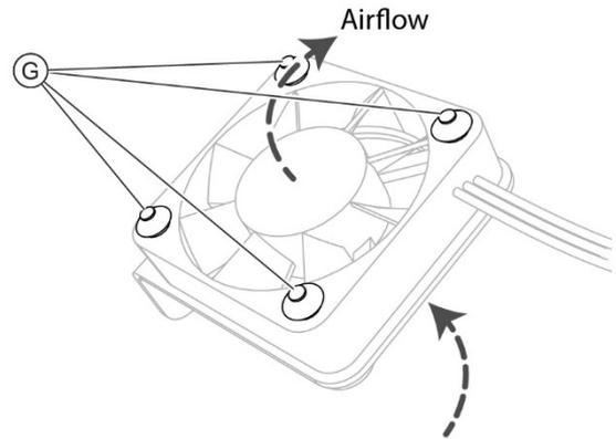
Fig. 118 - Insert the anti-vibration supports
