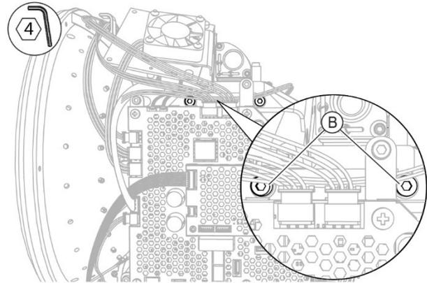
Fig. 90 - Loosen the screws
