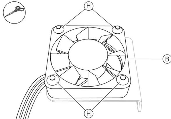
Fig. 106 - Cut the anti-vibration supports and remove the fan
