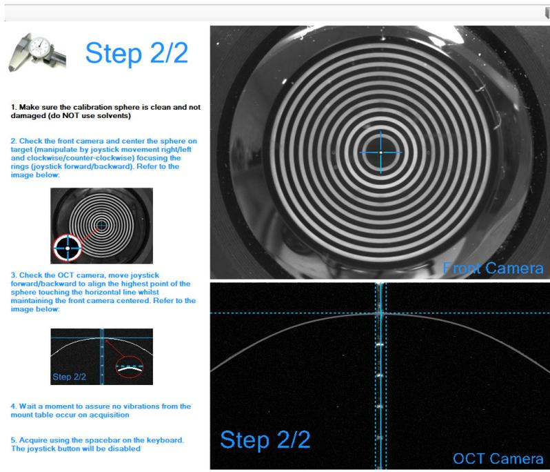
Fig. 52 - Curvature calibration Step 2/2
