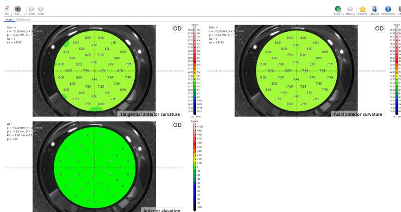
Fig. 53 - Acquisition of a 8mm calibration sphere
