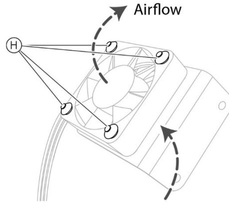
Fig. 108 - Insert the anti-vibration supports
