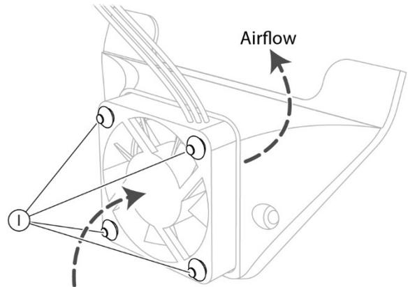
Fig. 96 - Insert the anti-vibration supports
