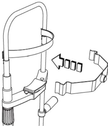
Fig. 48 - Place the calibration tool
