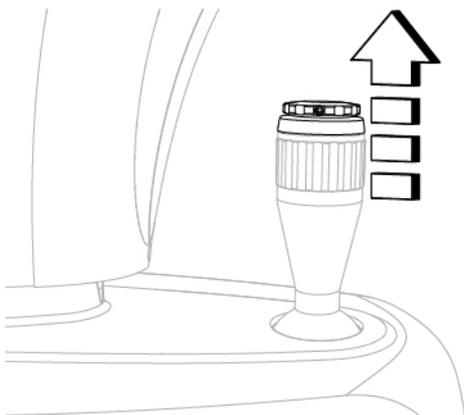
Fig. 82 - Remove the joystick button
