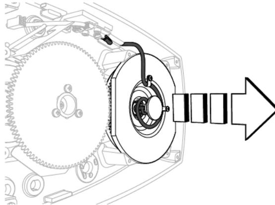
Fig. 80 - Remove the joystick
