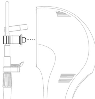
Fig. 49 - Align the calibration tool
