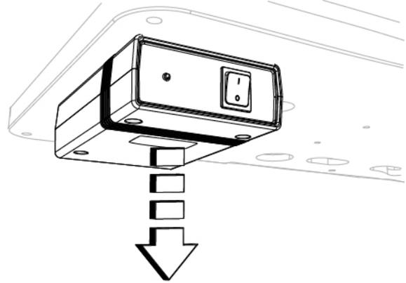
Fig. 56 - Remove the power supply unit
