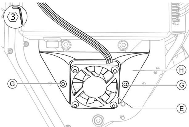
Fig. 97 - Place the cooling fan with the support
