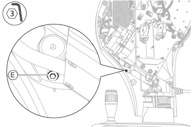
Fig. 63 - Unscrew the screw
