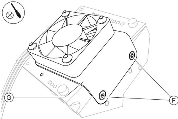
Fig. 105 - Unscrew the screws and remove the support
