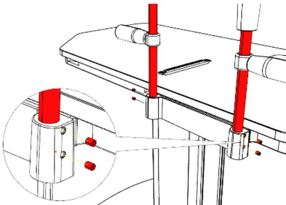
Fig. 19 - Loosen the grub screws of the chin rest
