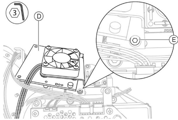
Fig. 104 - Unscrew the screw and remove the assembly
