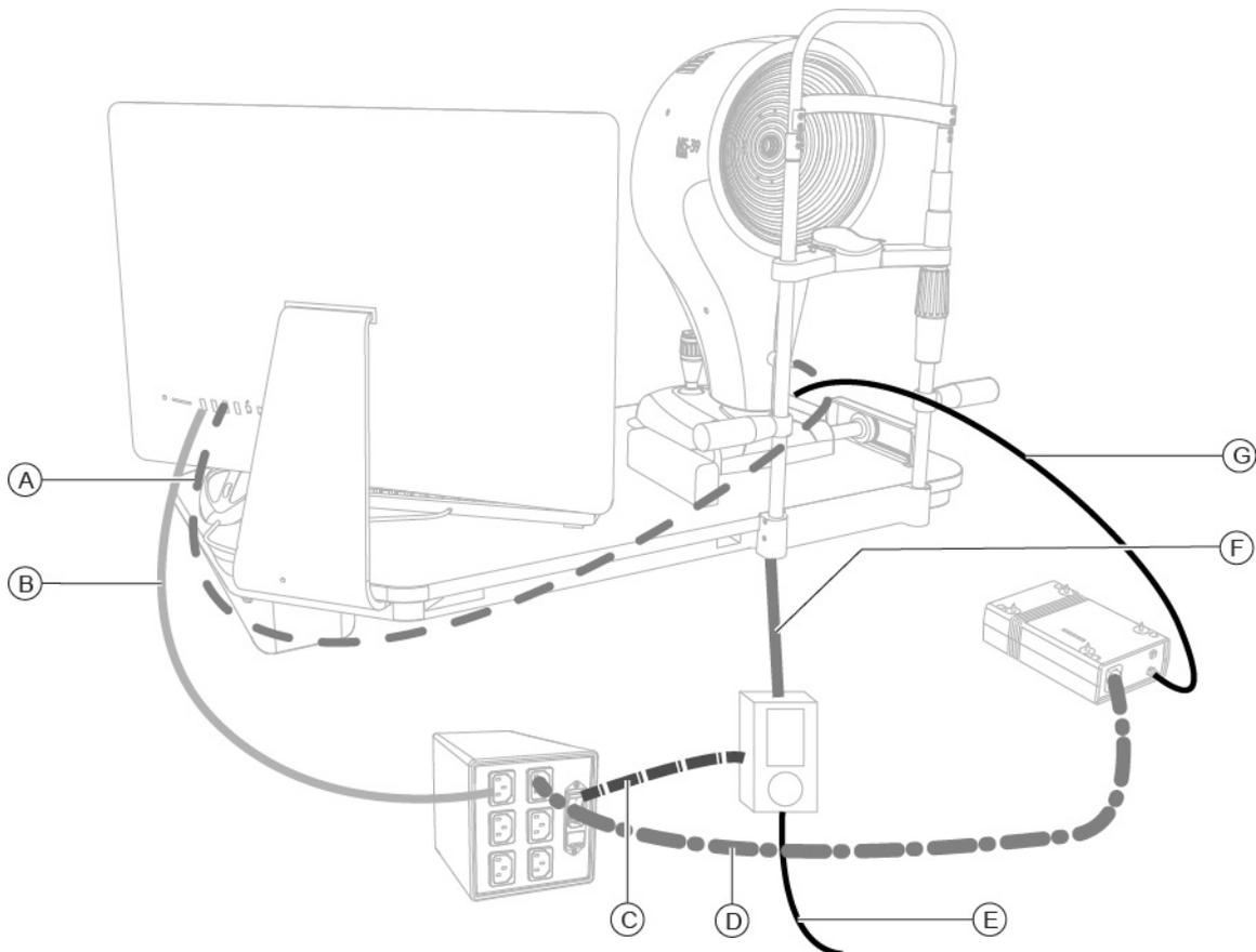
Fig. 123 - Connect the tester inside the patient area
