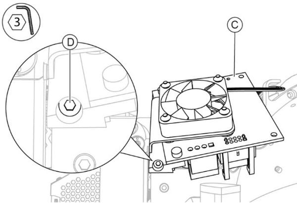
Fig. 121 - Install the assembly
