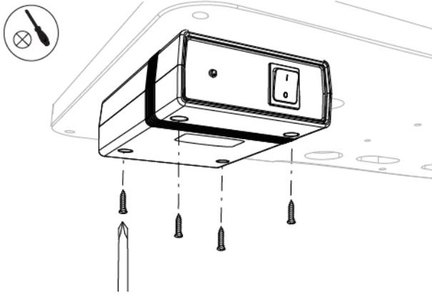
Fig. 55 - Unscrew the screws
