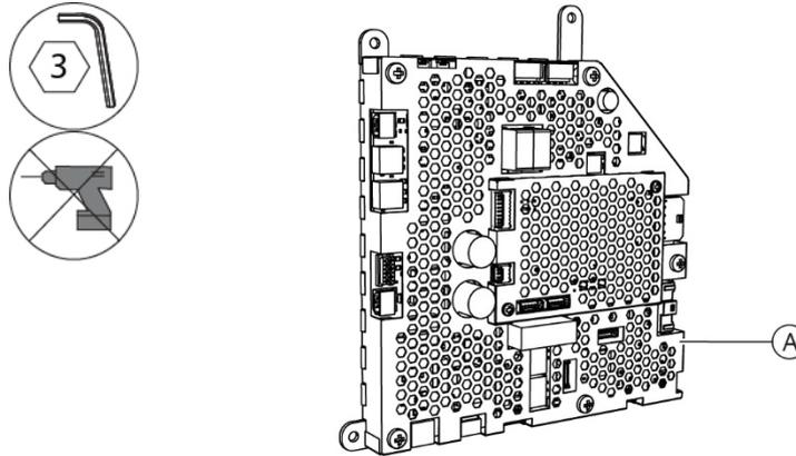
Fig. 84 - Power Supply circuit board
