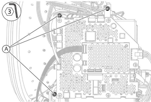
Fig. 101 - Tighten the screws
