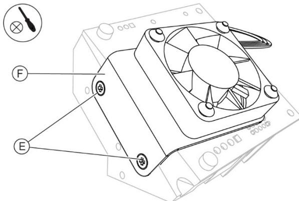
Fig. 119 - Place the support and screw in the screws
