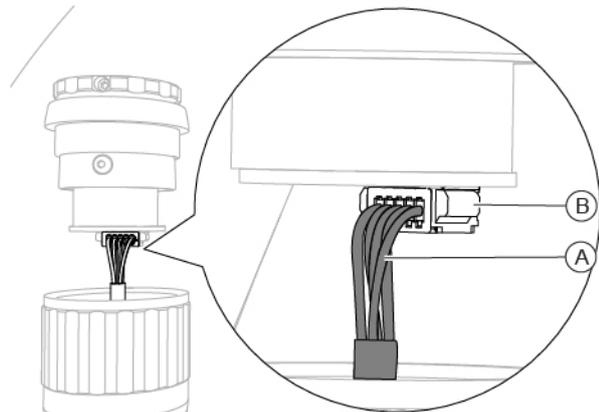
Fig. 83 - Disconnect the cable
