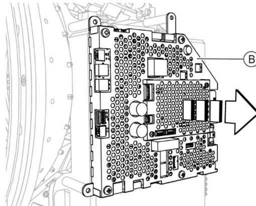
Fig. 87 - Remove the Power Supply circuit board
