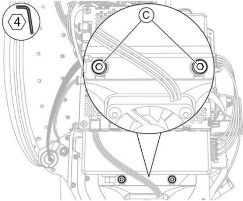
Fig. 99 - Tighten the screws
