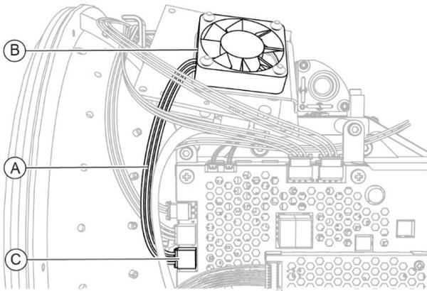
Fig. 103 - Disconnect the connection cable
