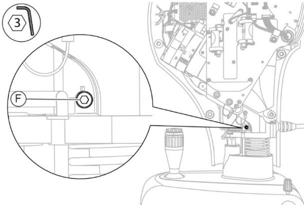
Fig. 64 - Unscrew the screw
